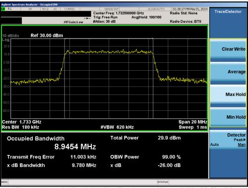
Plot 6-12. Occupied Bandwidth Plot (Band 4 – 10.0MHz 16-QAM – RB Size 50)
