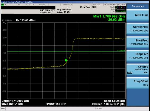
Plot 6-53. Lower Band Edge Plot (Band 4 – 5.0MHz QPSK – RB Size 25)
