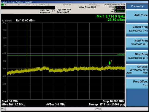
Plot 6-29. Conducted Spurious Plot (Band 4 – 5.0MHz QPSK – RB Size 1, RB Offset 0 – Low Channel)
