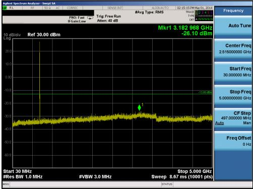
Plot 6-21. Conducted Spurious Plot (Band 17 – 10.0MHz QPSK – RB Size 1, RB Offset 0 – High Channel)
