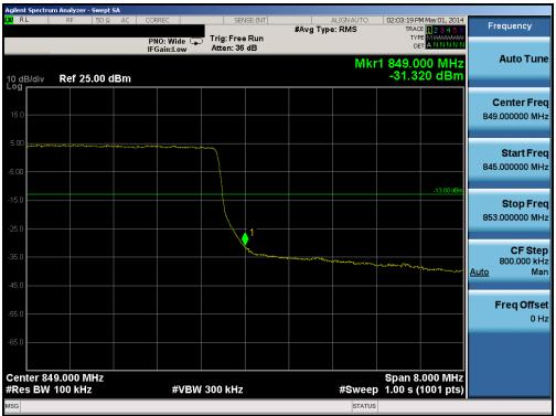
Plot 6-52. Upper Band Edge Plot (Band 5 – 10.0MHz QPSK – RB Size 50)
