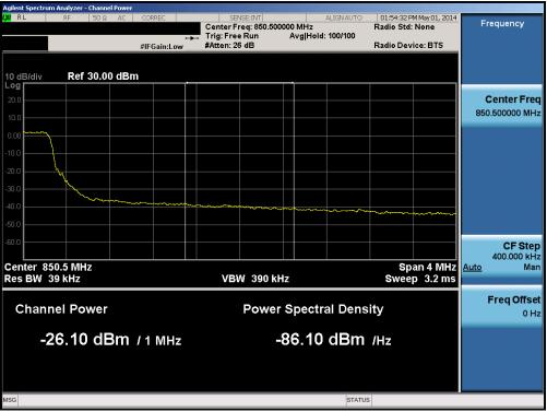
Plot 6-50. Upper Extended Band Edge Plot (Band 5 – 5.0MHz QPSK – RB Size 25)
