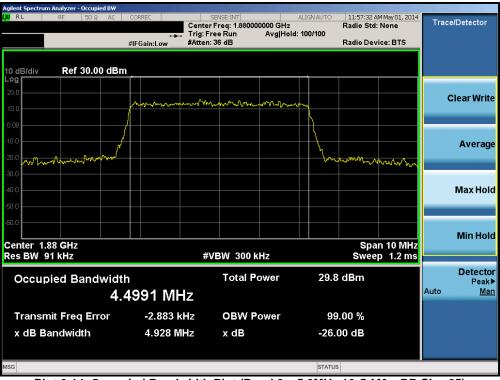
Plot 6-14. Occupied Bandwidth Plot (Band 2 - 5.0MHz 16-QAM - RB Size 25)
