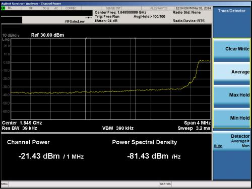
Plot 6-62. Lower Extended Band Edge Plot (Band 2 – 5.0MHz QPSK – RB Size 25)
