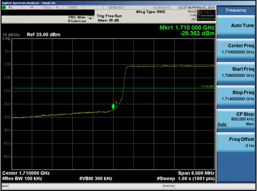
Plot 6-57. Lower Band Edge Plot (Band 4 – 10.0MHz QPSK – RB Size 50)
