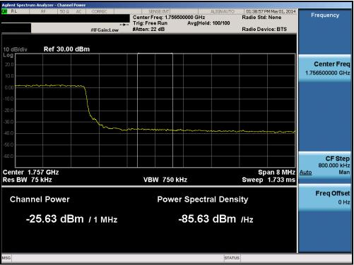
Plot 6-60. Upper Extended Band Edge Plot (Band 4 – 10.0MHz QPSK – RB Size 50)
