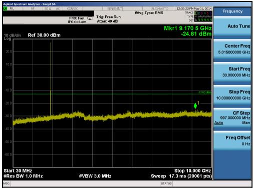
Plot 6-39. Conducted Spurious Plot (Band 2 – 5.0MHz QPSK – RB Size 1, RB Offset 0 – High Channel)
