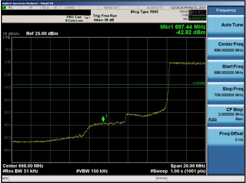
Plot 6-41. Lower Band Edge Plot (Band 17 – 5.0MHz QPSK – RB Size 25)
