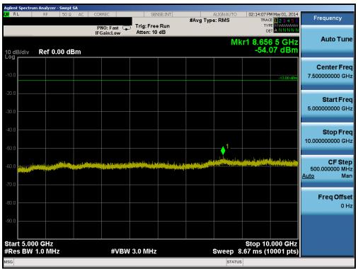
Plot 6-18. Conducted Spurious Plot (Band 17 – 10.0MHz QPSK – RB Size 1, RB Offset 0 – Low Channel)
