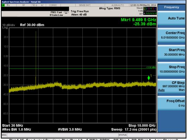
Plot 6-35. Conducted Spurious Plot (Band 2 – 5.0MHz QPSK – RB Size 1, RB Offset 0 – Low Channel)
