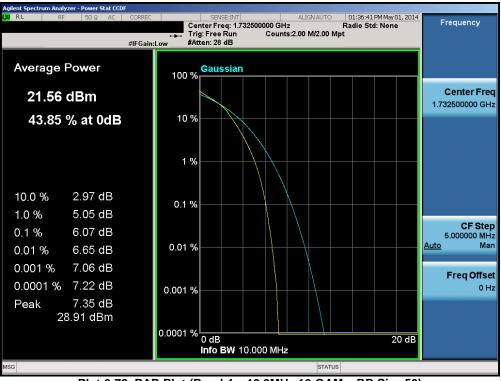
Plot 6-72. PAR Plot (Band 4 - 10.0MHz 16-QAM - RB Size 50)
