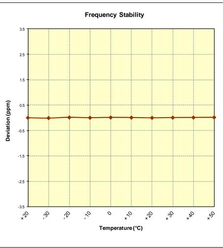
Figure 6-10. Frequency Stability Graph (Band 2)
