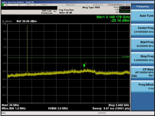
Plot 6-27. Conducted Spurious Plot (Band 5 – 10.0MHz QPSK – RB Size 1, RB Offset 0 – High Channel)
