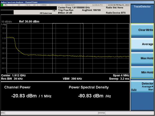
Plot 6-64. Upper Extended Band Edge Plot (Band 2 – 5.0MHz QPSK – RB Size 25)
