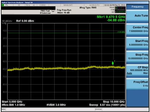
Plot 6-28. Conducted Spurious Plot (Band 5 – 10.0MHz QPSK – RB Size 1, RB Offset 0 – High Channel)
