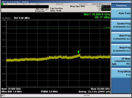
Plot 6-40. Conducted Spurious Plot (Band 2 – 5.0MHz QPSK – RB Size 1, RB Offset 0 – High Channel)
