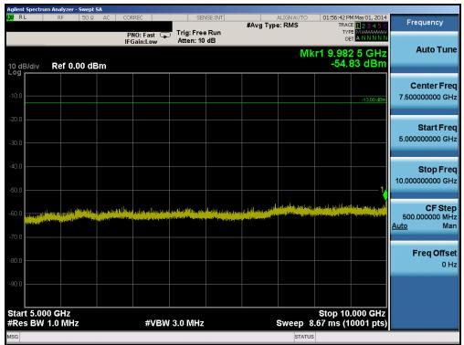
Plot 6-26. Conducted Spurious Plot (Band 5 – 10.0MHz QPSK – RB Size 1, RB Offset 0 – Mid Channel)
