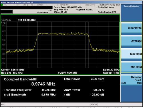
Plot 6-8. Occupied Bandwidth Plot (Band 5 – 10.0MHz 16-QAM – RB Size 50)
