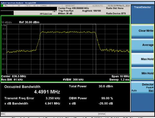
Plot 6-6. Occupied Bandwidth Plot (Band 5 – 5.0MHz 16-QAM – RB Size 25)
