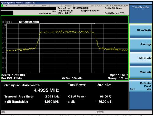
Plot 6-10. Occupied Bandwidth Plot (Band 4 - 5.0MHz 16-QAM - RB Size 25)
