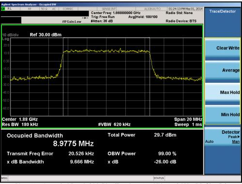
Plot 6-16. Occupied Bandwidth Plot (Band 2 - 10.0MHz 16-QAM - RB Size 50)
