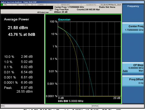
Plot 6-70. PAR Plot (Band 4 – 5.0MHz 16-QAM – RB Size 25)
