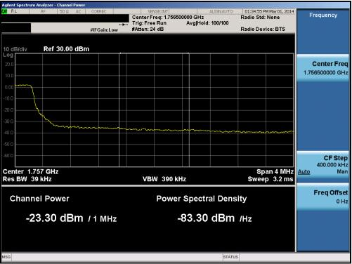
Plot 6-56. Upper Extended Band Edge Plot (Band 4 – 5.0MHz QPSK – RB Size 25)
