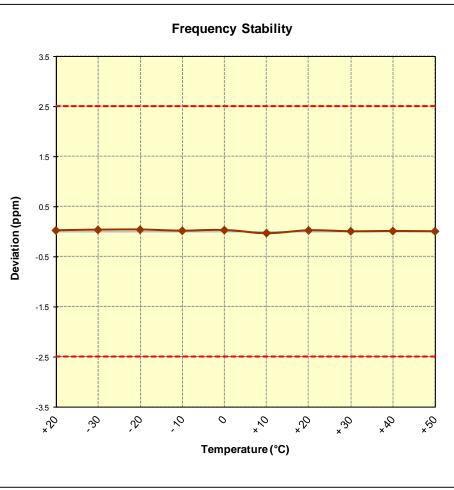
Figure 6-7. Frequency Stability Graph (Band 17)
