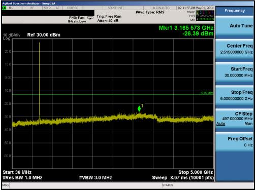
Plot 6-19. Conducted Spurious Plot (Band 17 – 10.0MHz QPSK – RB Size 1, RB Offset 0 – Mid Channel)
