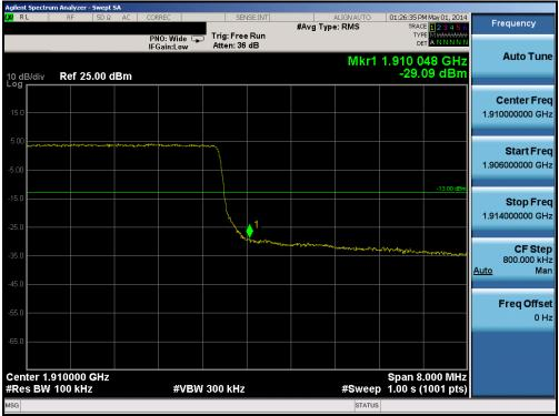
Plot 6-67. Upper Band Edge Plot (Band 2 – 10.0MHz QPSK – RB Size 50)
