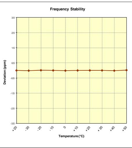
Figure 6-9. Frequency Stability Graph (Band 4)
