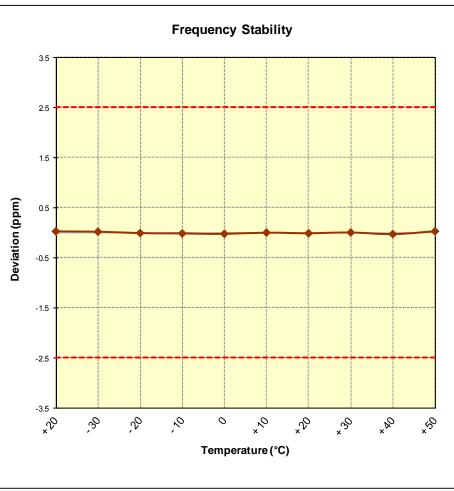
Figure 6-8. Frequency Stability Graph (Band 5)
