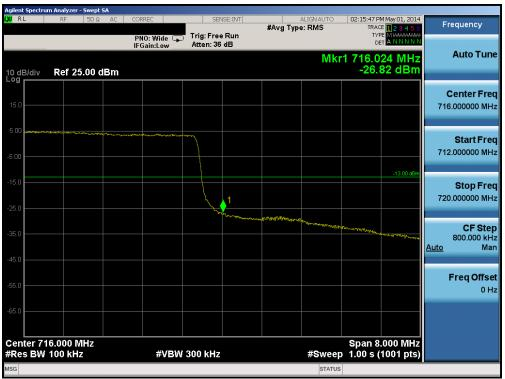
Plot 6-46. Upper Band Edge Plot (Band 17 – 10.0MHz QPSK – RB Size 50)
