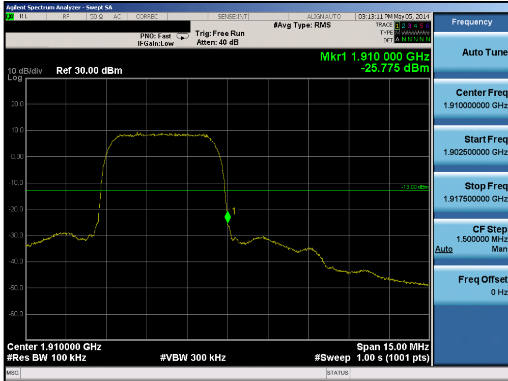
Plot 6-19. Band Edge Plot (PCS WCDMA Mode – Ch. 9538)
