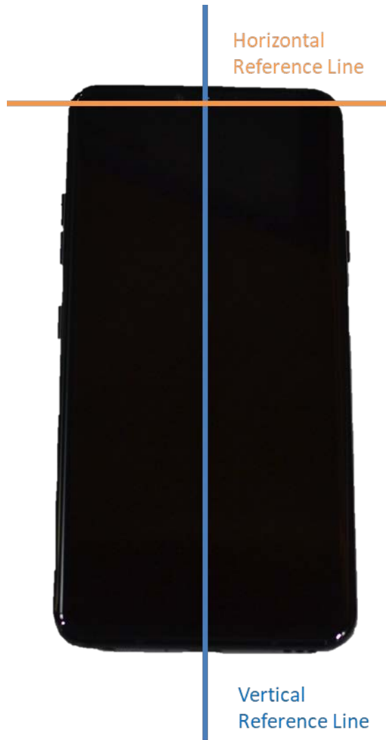
SAR Test Setup Photo 18 – Horizontal and Vertical Reference Lines
