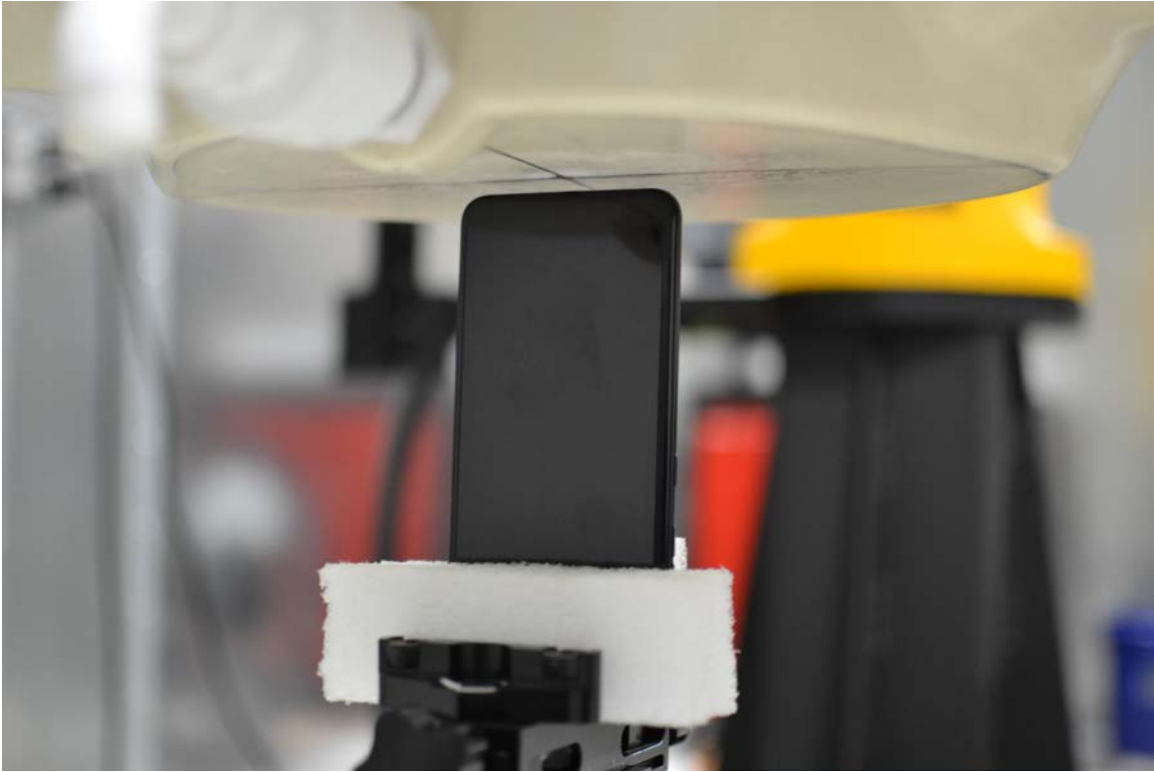
SAR Test Setup Photo 13 – Bottom Edge at 3 mm
