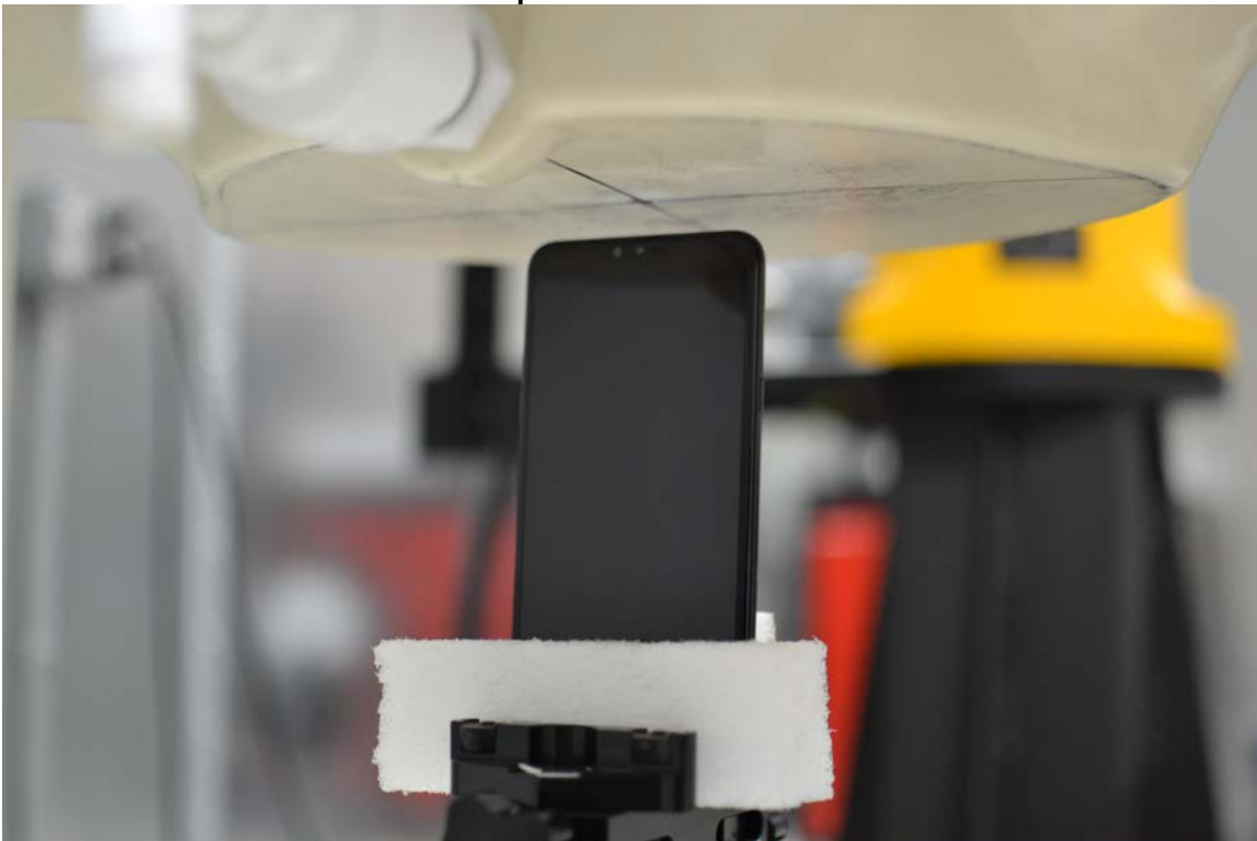
SAR Test Setup Photo 10 – Top Edge at 10 mm
