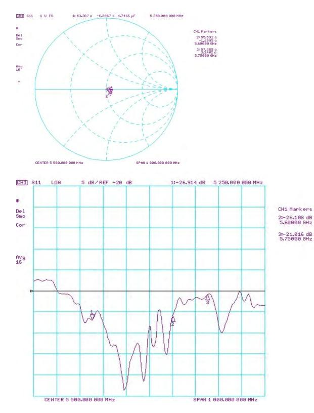
Impedance & Return-Loss Measurement Plot for Head TSL
