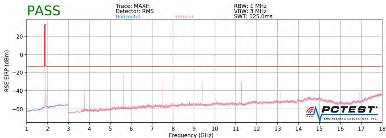
Plot 7-385. Radiated Spurious Plot above 1GHz (Band 2/25)
