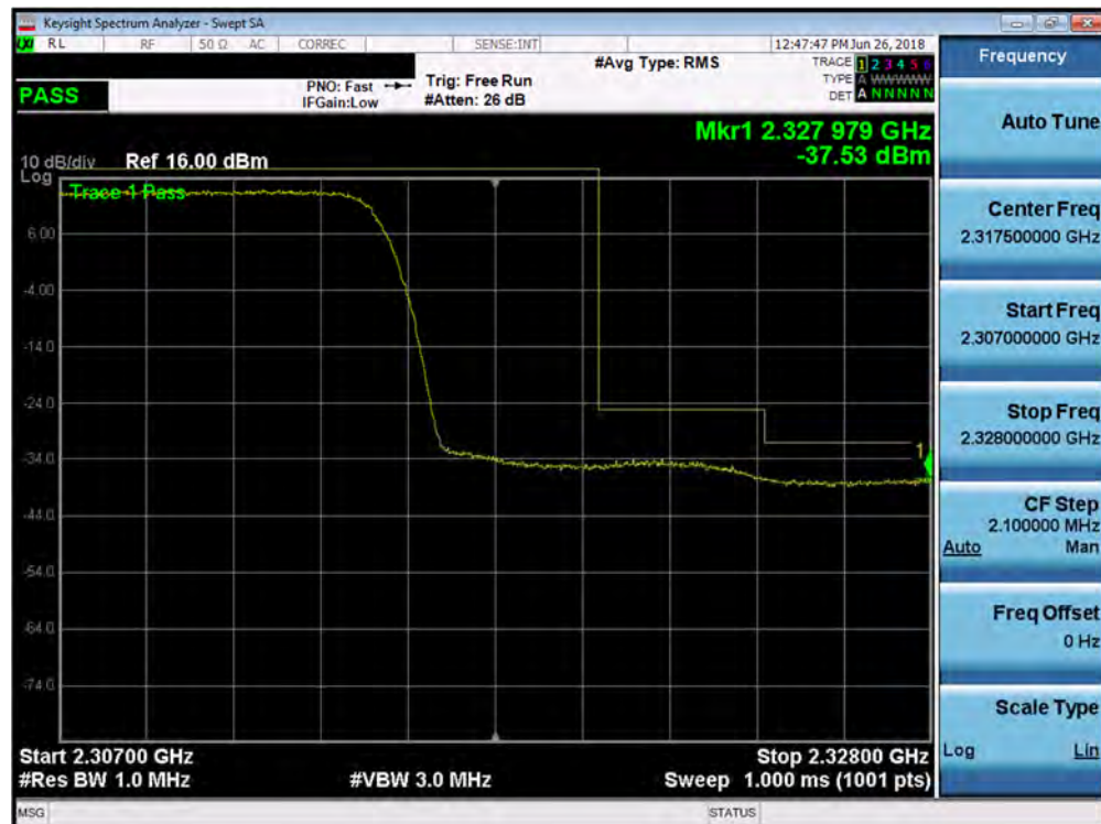
Plot 7-316. Upper Extended Band Edge Plot A (Band 30 - 10.0MHz QPSK - Full RB Configuration)
