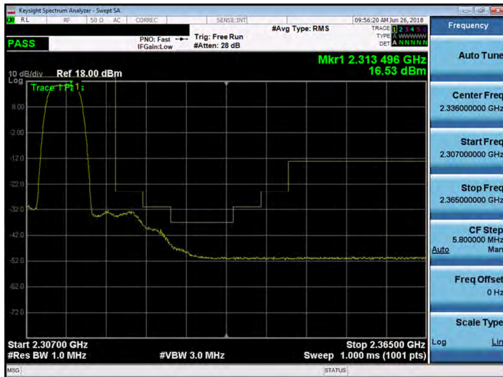
Plot 7-312. Upper Extended Band Edge Plot (Band 30 - 5.0MHz QPSK - Full RB Configuration)
