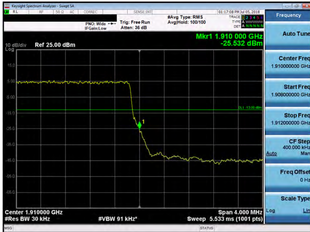
Plot 7-281. Upper Band Edge Plot (Band 2 - 3.0MHz QPSK - Full RB Configuration)
