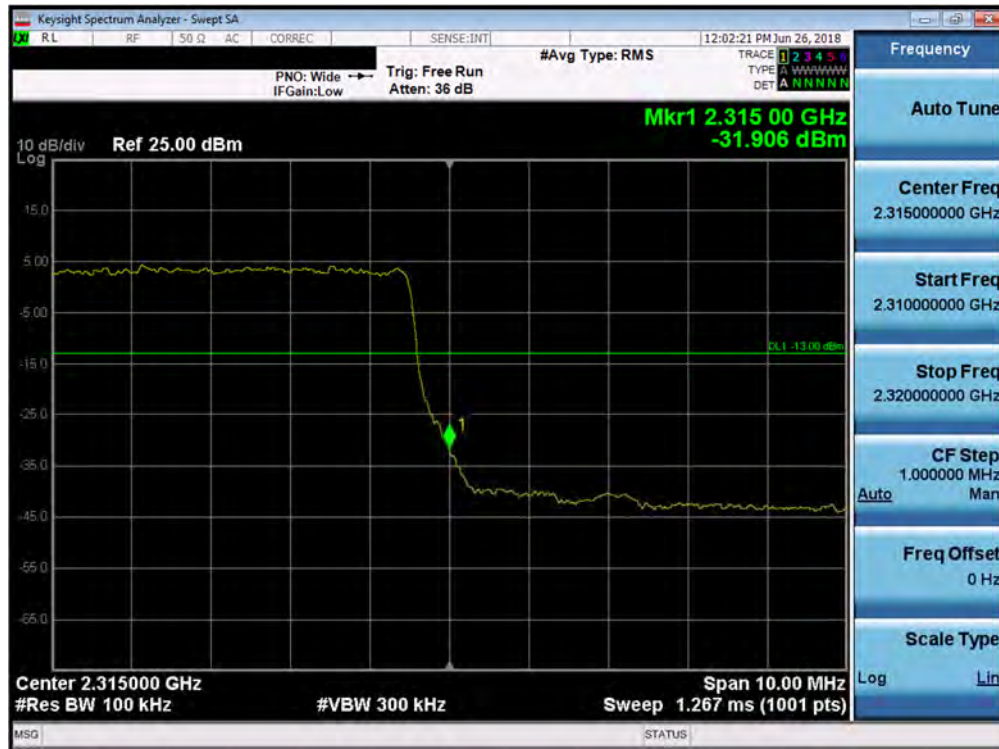
Plot 7-315. Upper Band Edge Plot (Band 30 - 10.0MHz QPSK - Full RB Configuration)
