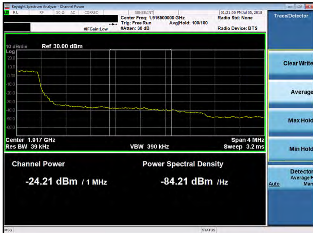
Plot 7-284. Upper Extended Band Edge Plot (Band 25 - 3.0MHz QPSK - Full RB Configuration)
