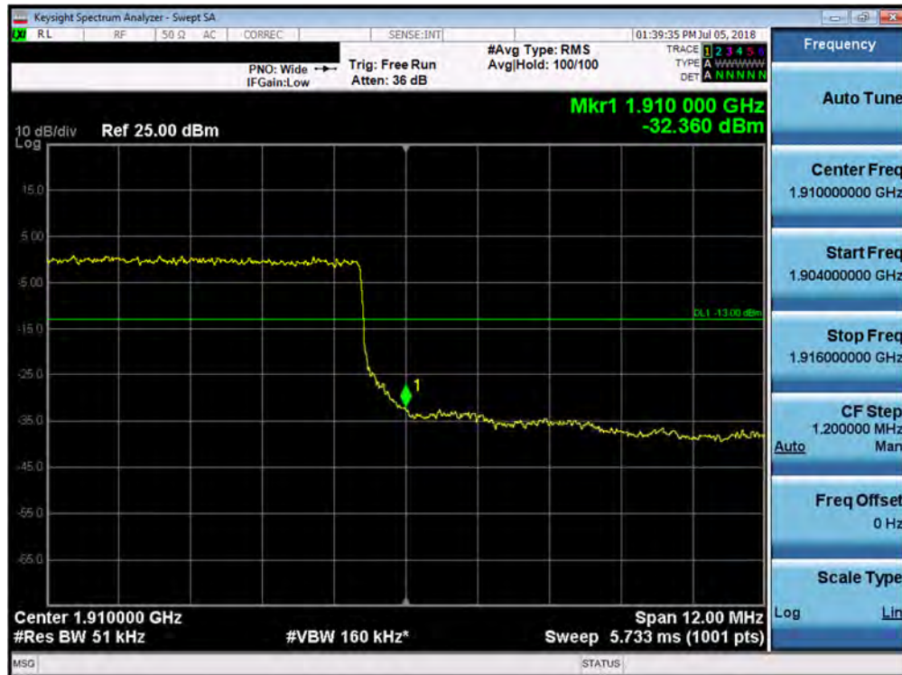
Plot 7-299. Upper Band Edge Plot (Band 2 - 15.0MHz QPSK - Full RB Configuration)
