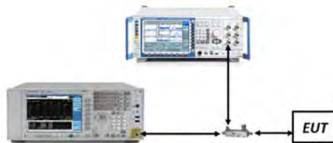
Figure 7-6. Test Instrument & Measurement Setup
