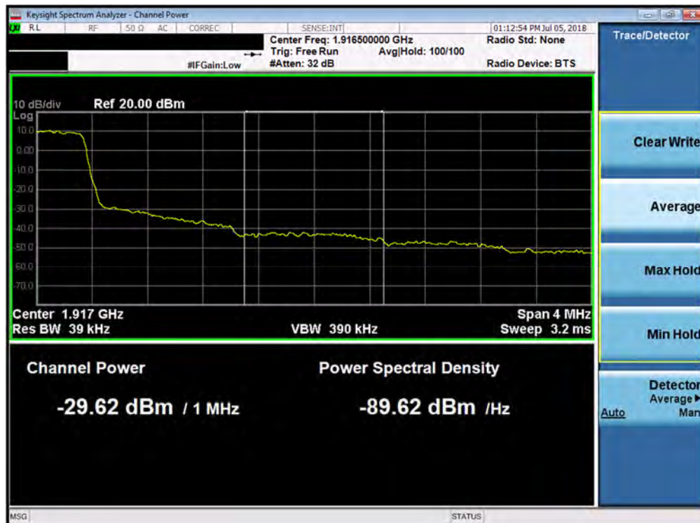
Plot 7-278. Upper Extended Band Edge Plot (Band 25 - 1.4MHz QPSK - Full RB Configuration)
