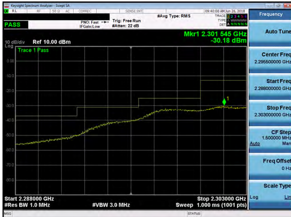
Plot 7-310. Lower Extended Band Edge Plot (Band 30 - 5.0MHz QPSK - Full RB Configuration)
