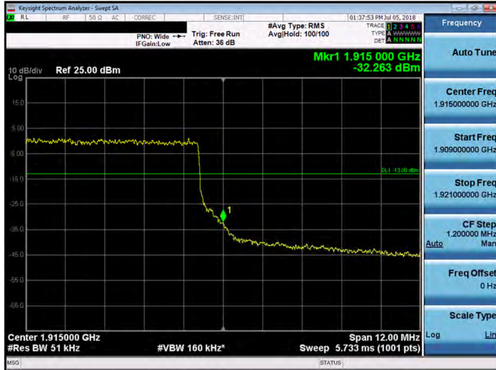
Plot 7-301. Upper Band Edge Plot (Band 25 - 15.0MHz QPSK - Full RB Configuration)
