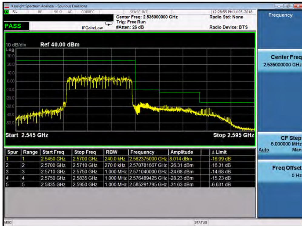
Plot 7-327. Upper ACP Plot (Band 7 - 15.0MHz QPSK - RB Size 75)
