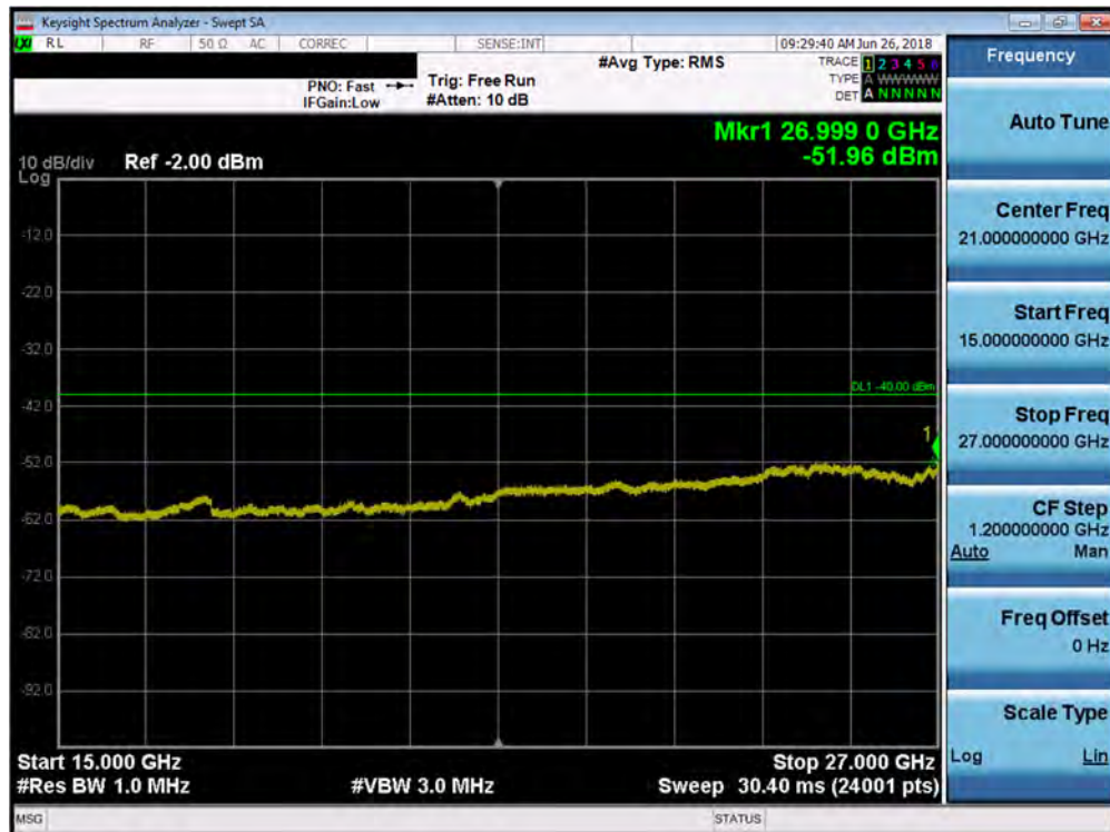
Plot 7-171. Conducted Spurious Plot (Band 30 - 5.0MHz QPSK - RB Size 1, RB Offset 0 - Mid Channel)
