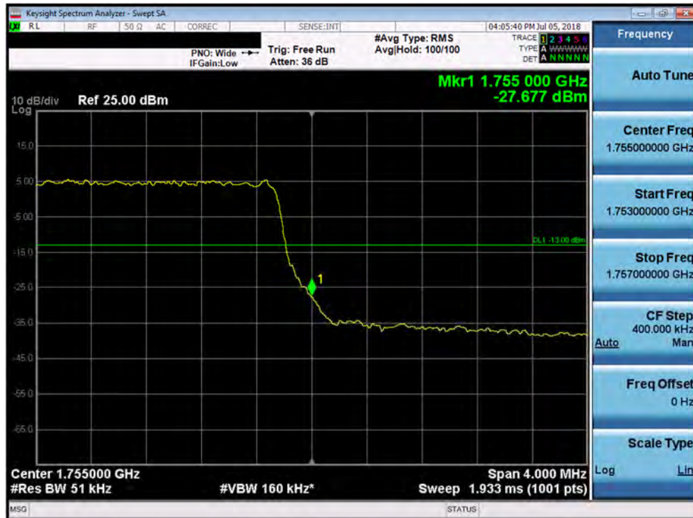
Plot 7-251. Upper Band Edge Plot (Band 4 - 5.0MHz QPSK - Full RB Configuration)
