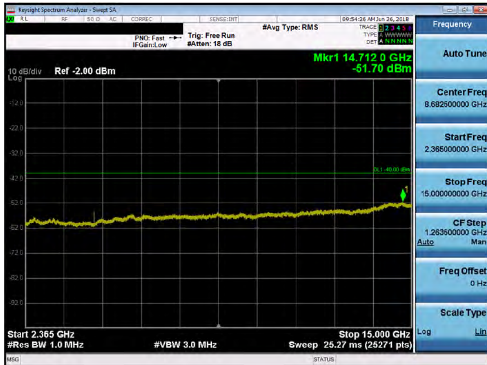
Plot 7-173. Conducted Spurious Plot (Band 30 - 5.0MHz QPSK - RB Size 1, RB Offset 0 - High Channel)
