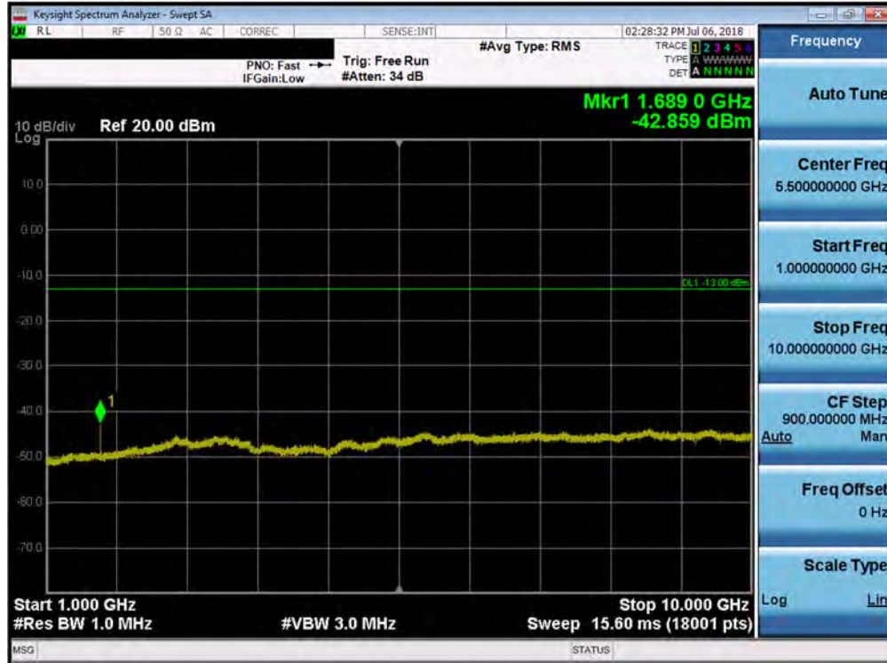
Plot 7-147. Conducted Spurious Plot (Band 26/5 - 5.0MHz QPSK - RB Size 1, RB Offset 0 - High Channel)
