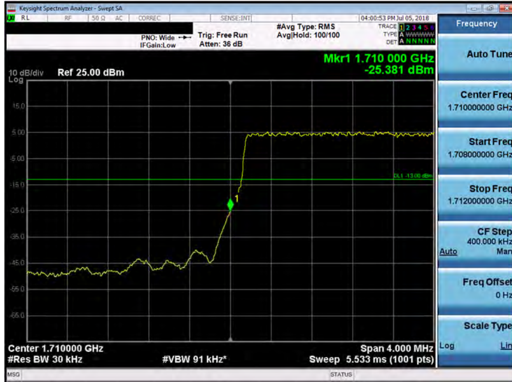
Plot 7-243. Lower Band Edge Plot (Band 66/4 - 3.0MHz QPSK - Full RB Configuration)
