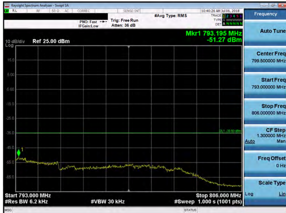
Plot 7-226. Upper Band Edge Plot (Band 13 - 10.0MHz QPSK - Full RB Configuration)
