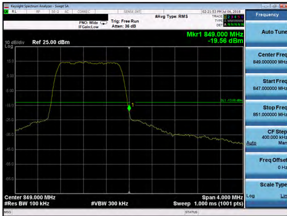
Plot 7-228. Upper Band Edge Plot (Band 26/5 - 1.4MHz QPSK - Full RB Configuration)
