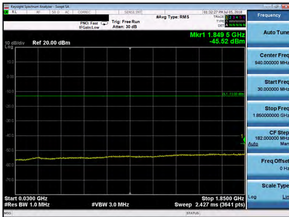
Plot 7-160. Conducted Spurious Plot (Band 25/2 - 15.0MHz QPSK - RB Size 1, RB Offset 0 - Mid Channel)
