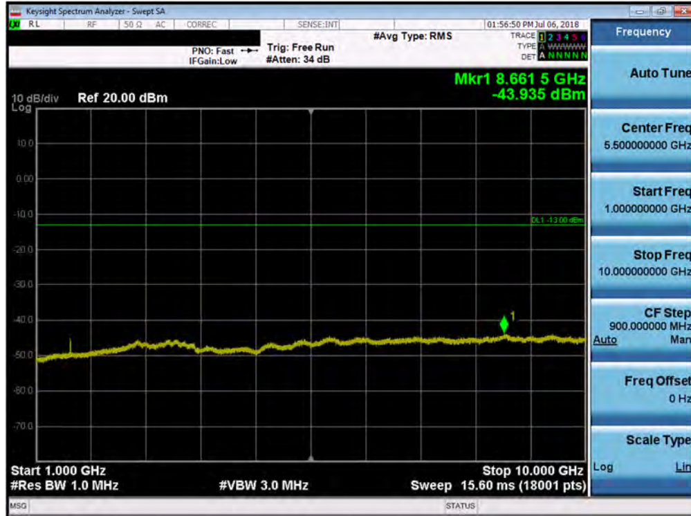
Plot 7-138. Conducted Spurious Plot (Band 13 - 5.0MHz QPSK - RB Size 1, RB Offset 0 - High Channel)
