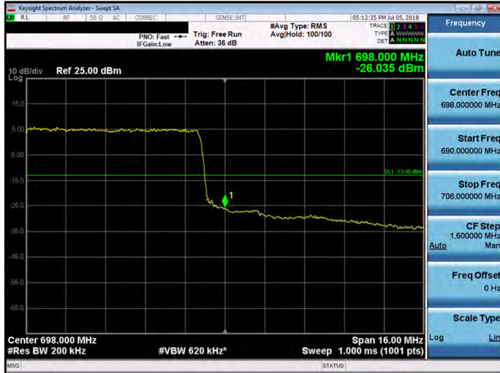
Plot 7-207. Upper Band Edge Plot (Band 71 - 20.0MHz QPSK - Full RB Configuration)
