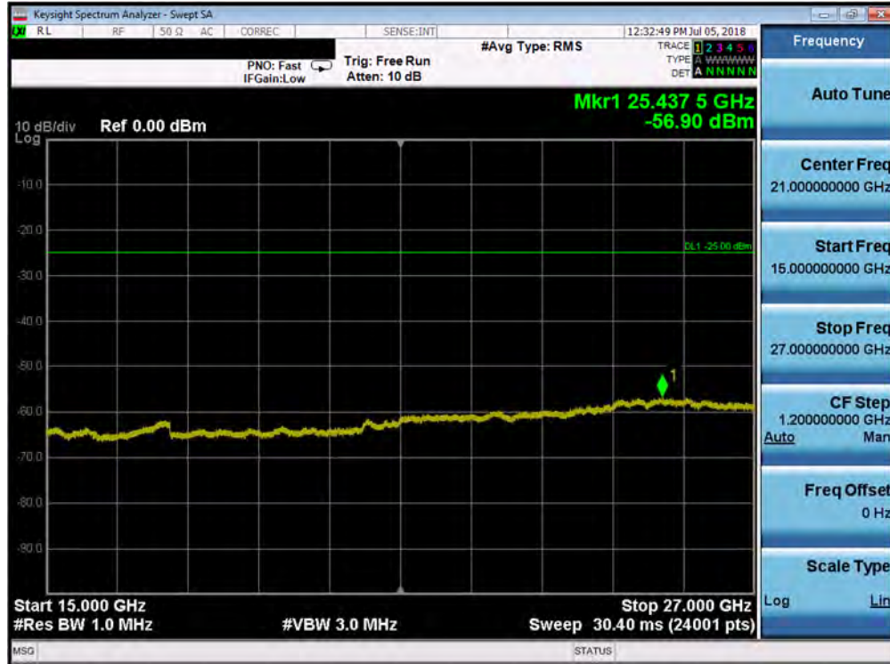
Plot 7-183. Conducted Spurious Plot (Band 7 - 20.0MHz QPSK - RB Size 1, RB Offset 0 - High Channel)
