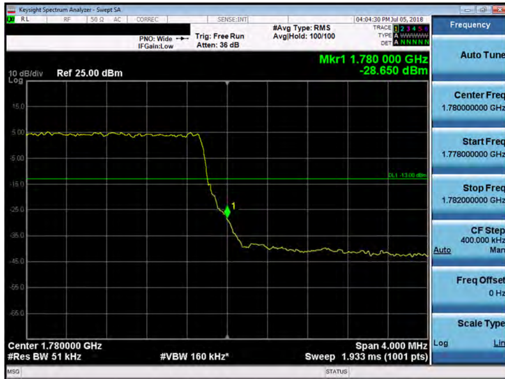
Plot 7-253. Upper Band Edge Plot (Band 66 - 5.0MHz QPSK - Full RB Configuration)
