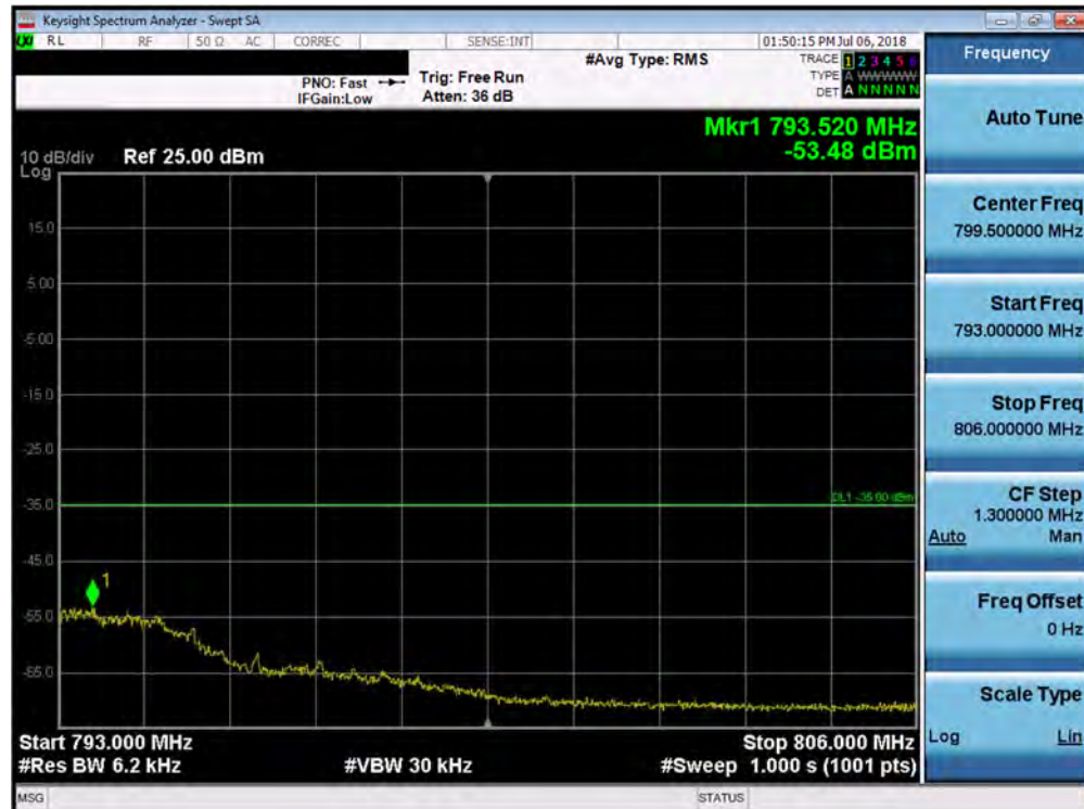
Plot 7-222. Upper Emission Mask (Band 13 - 5.0MHz QPSK - Full RB Configuration)
