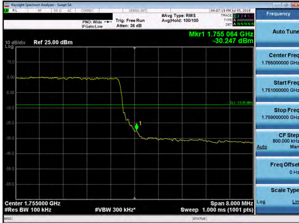
Plot 7-257. Upper Band Edge Plot (Band 4 - 10.0MHz QPSK - Full RB Configuration)
