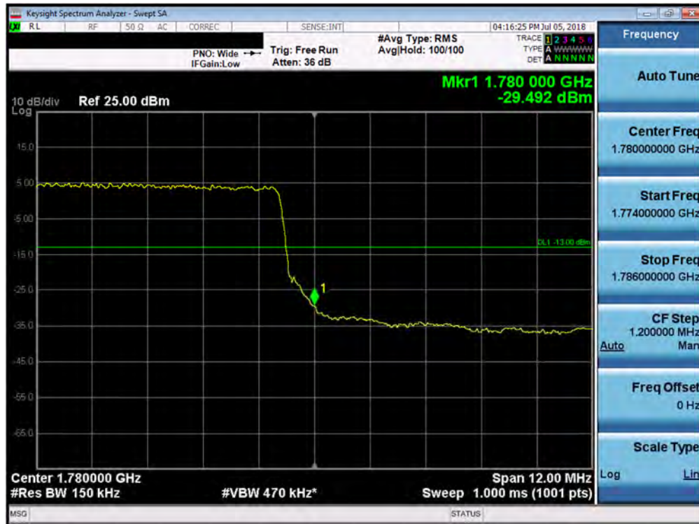
Plot 7-265. Upper Band Edge Plot (Band 66 - 15.0MHz QPSK - Full RB Configuration)
