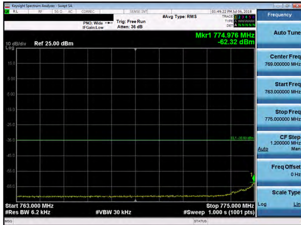
Plot 7-220. Lower Emission Mask (Band 13 - 5.0MHz QPSK - Full RB Configuration)
