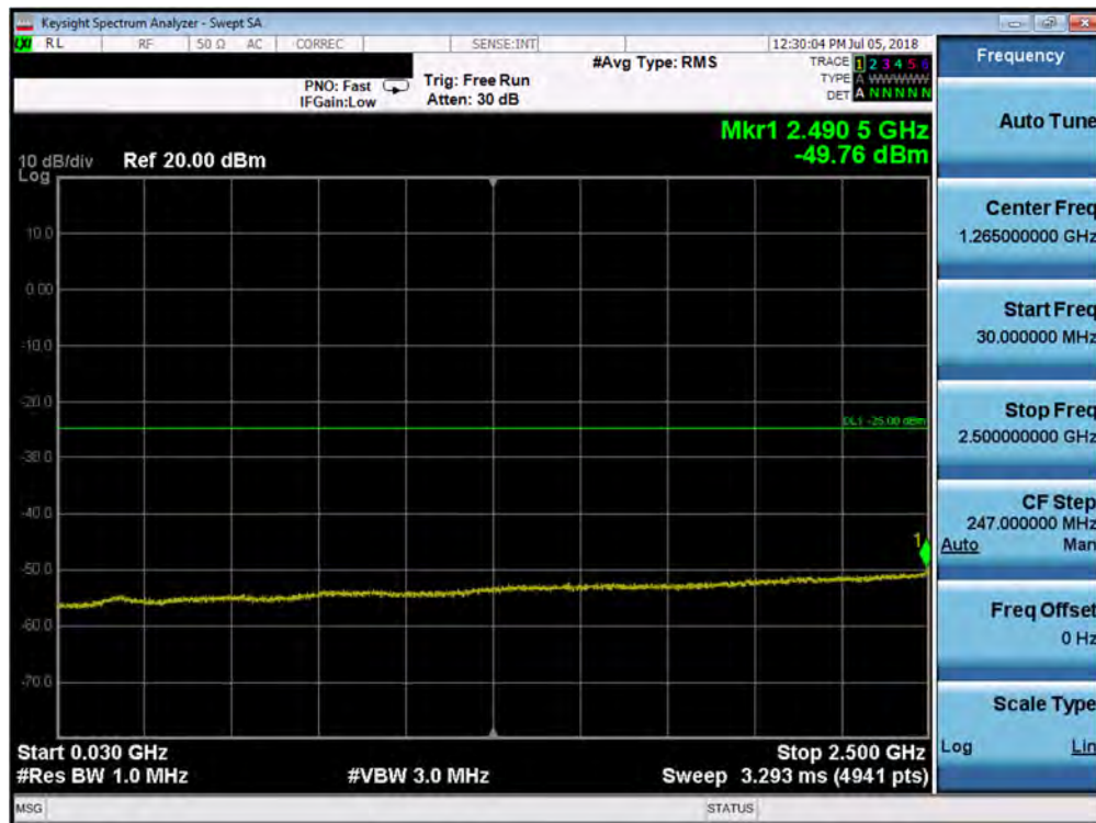
Plot 7-178. Conducted Spurious Plot (Band 7 - 20.0MHz QPSK - RB Size 1, RB Offset 0 - Mid Channel)
