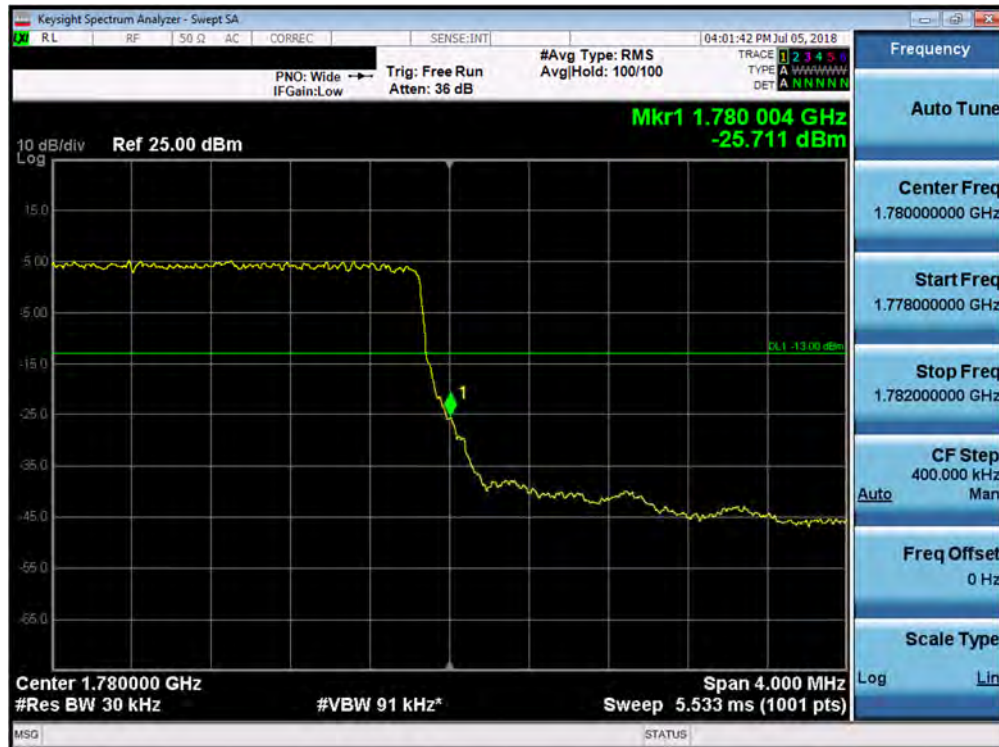
Plot 7-247. Upper Band Edge Plot (Band 66 - 3.0MHz QPSK - Full RB Configuration)
