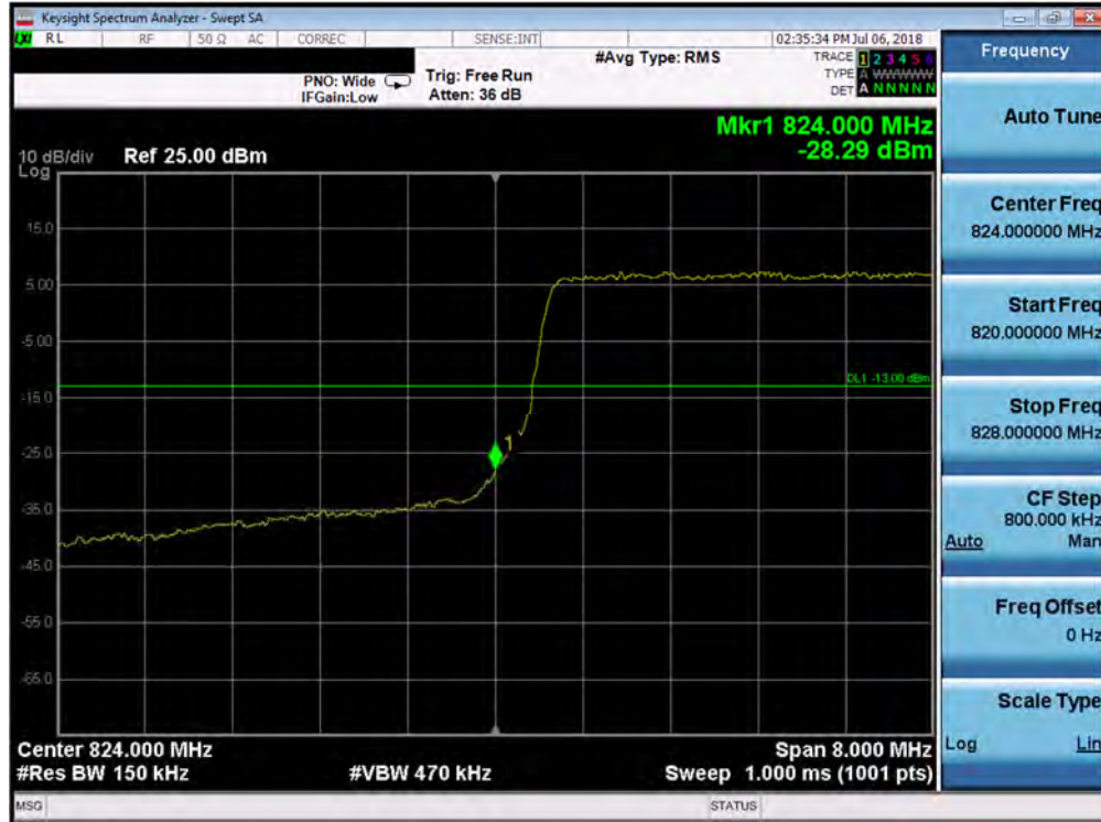
Plot 7-233. Lower Band Edge Plot (Band 26/5 - 10.0MHz QPSK - Full RB Configuration)
