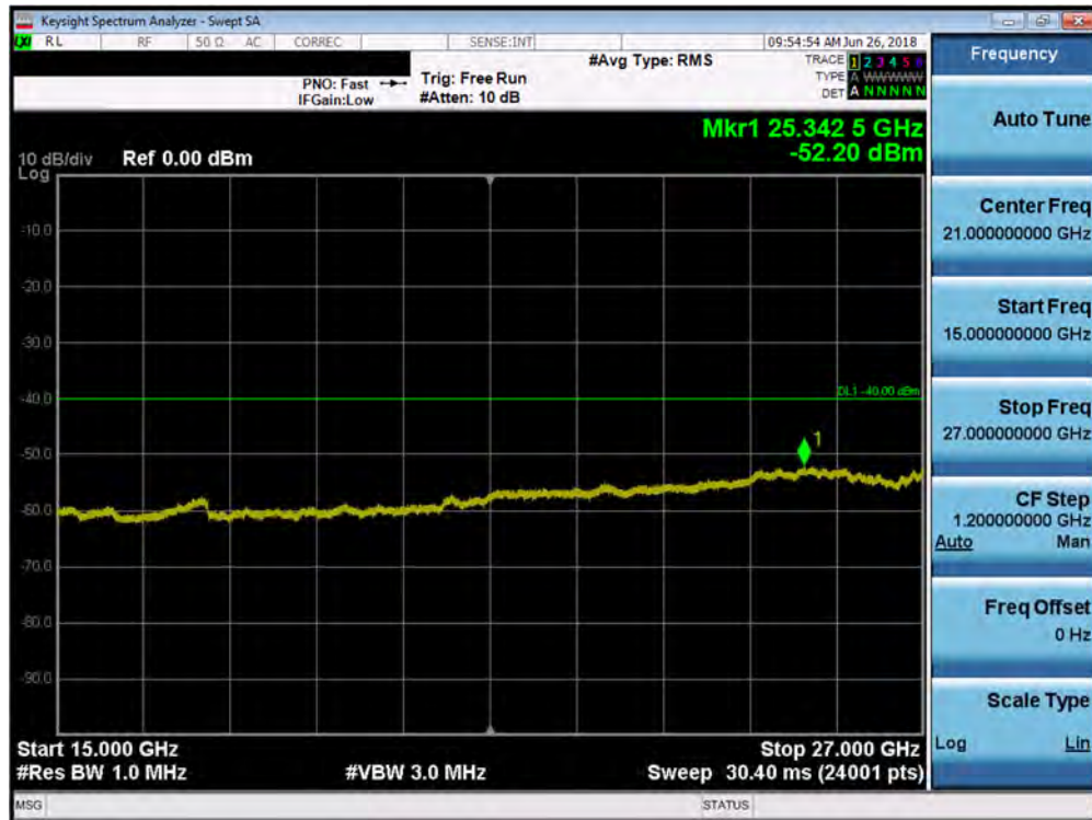
Plot 7-174. Conducted Spurious Plot (Band 30 - 5.0MHz QPSK - RB Size 1, RB Offset 0 - High Channel)
