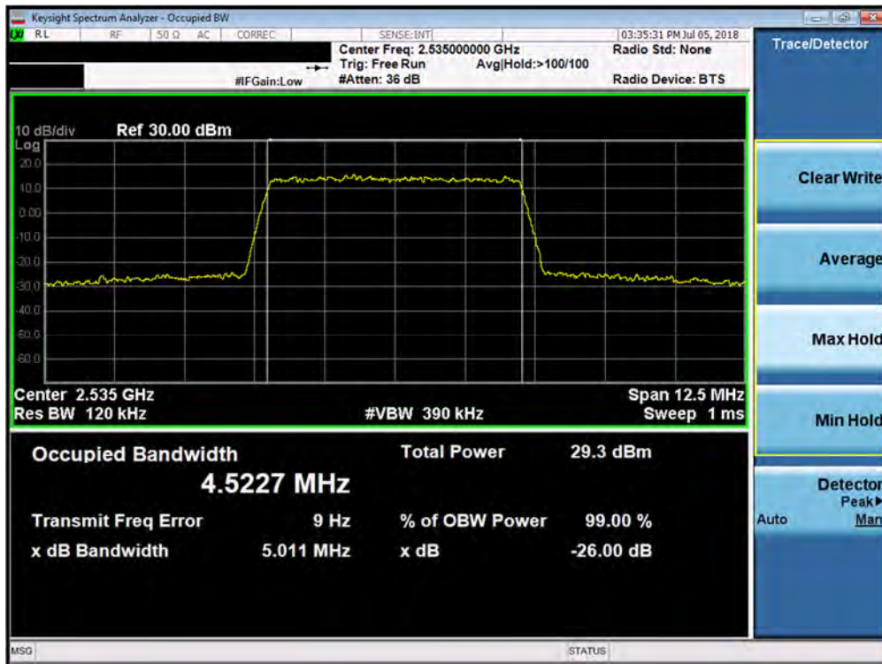
Plot 7-90. Occupied Bandwidth Plot (Band 7 - 5.0MHz 64-QAM - Full RB Configuration)
