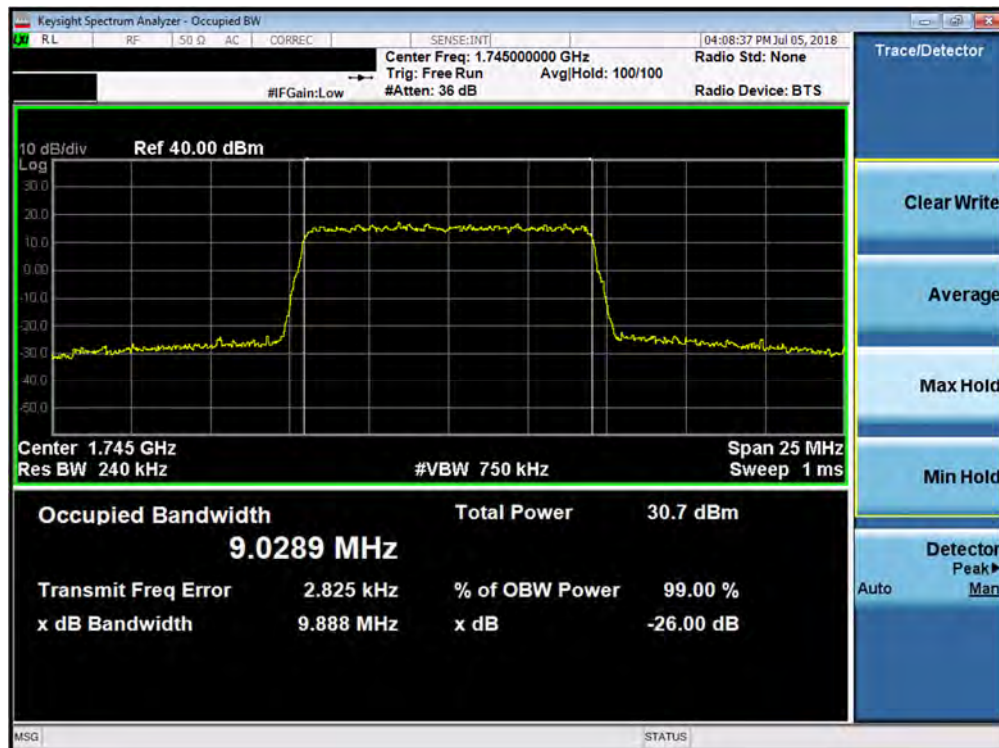
Plot 7-57. Occupied Bandwidth Plot (Band 66/4 - 10.0MHz 64-QAM - Full RB Configuration)
