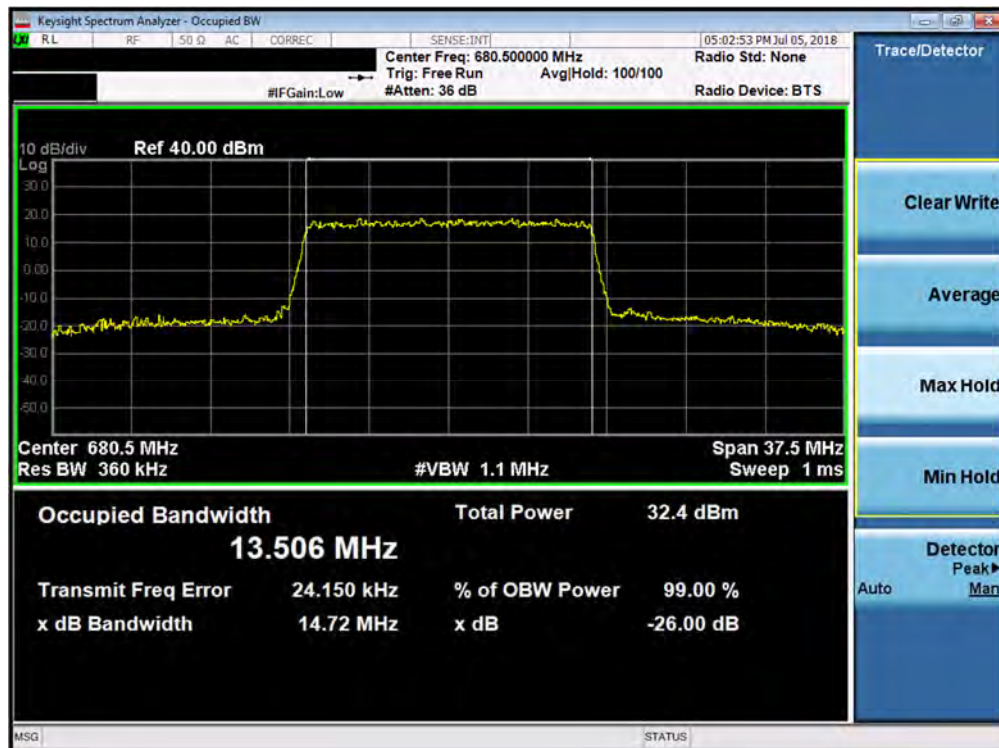
Plot 7-8. Occupied Bandwidth Plot (Band 71 - 15.0MHz 16-QAM - Full RB Configuration)
