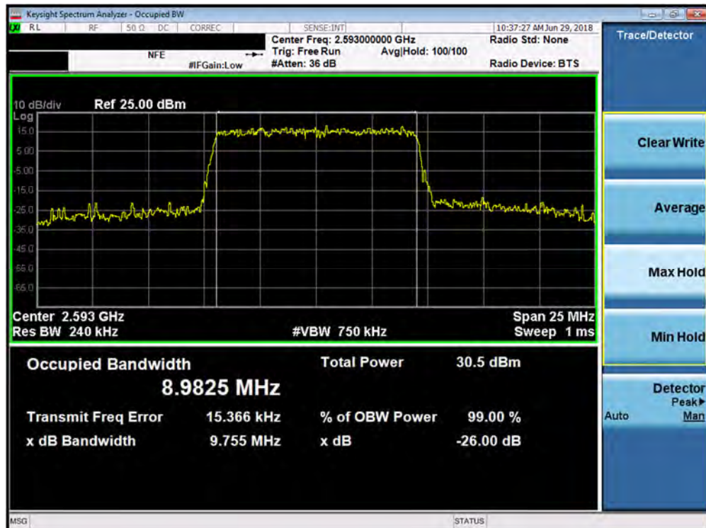
Plot 7-105. Occupied Bandwidth Plot (Band 41 - 10.0MHz 64-QAM - Full RB Configuration)
