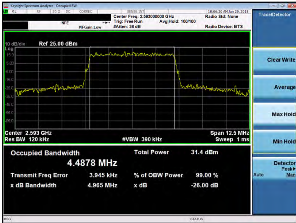
Plot 7-101. Occupied Bandwidth Plot (Band 41 - 5.0MHz 16-QAM - Full RB Configuration)
