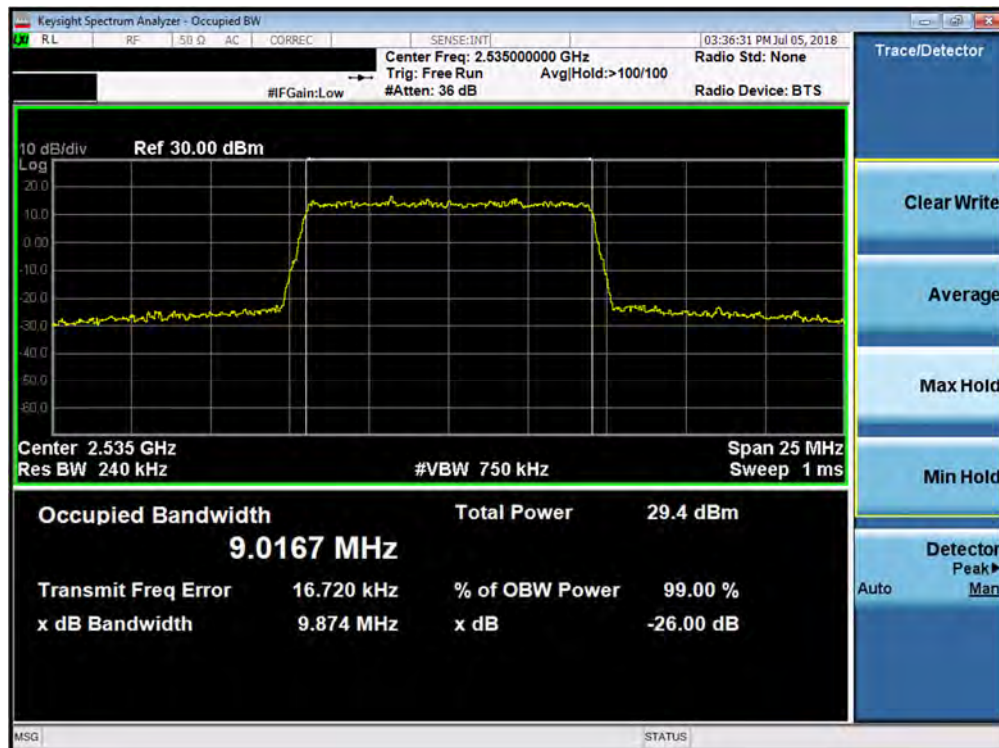
Plot 7-93. Occupied Bandwidth Plot (Band 7 - 10.0MHz 64-QAM - Full RB Configuration)
