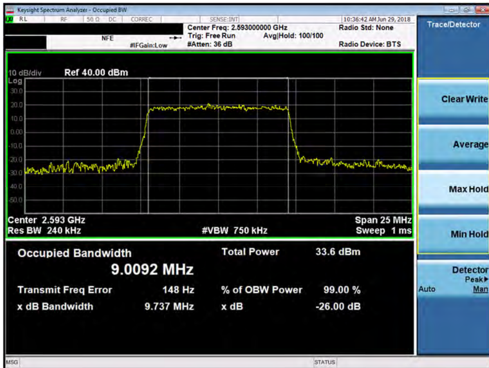
Plot 7-103. Occupied Bandwidth Plot (Band 41 - 10.0MHz QPSK - Full RB Configuration)
