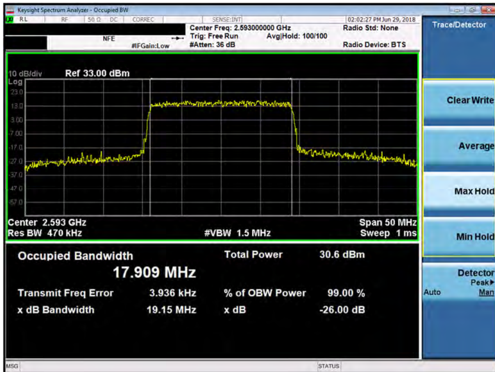
Plot 7-111. Occupied Bandwidth Plot (Band 41 - 20.0MHz 64-QAM - Full RB Configuration)
