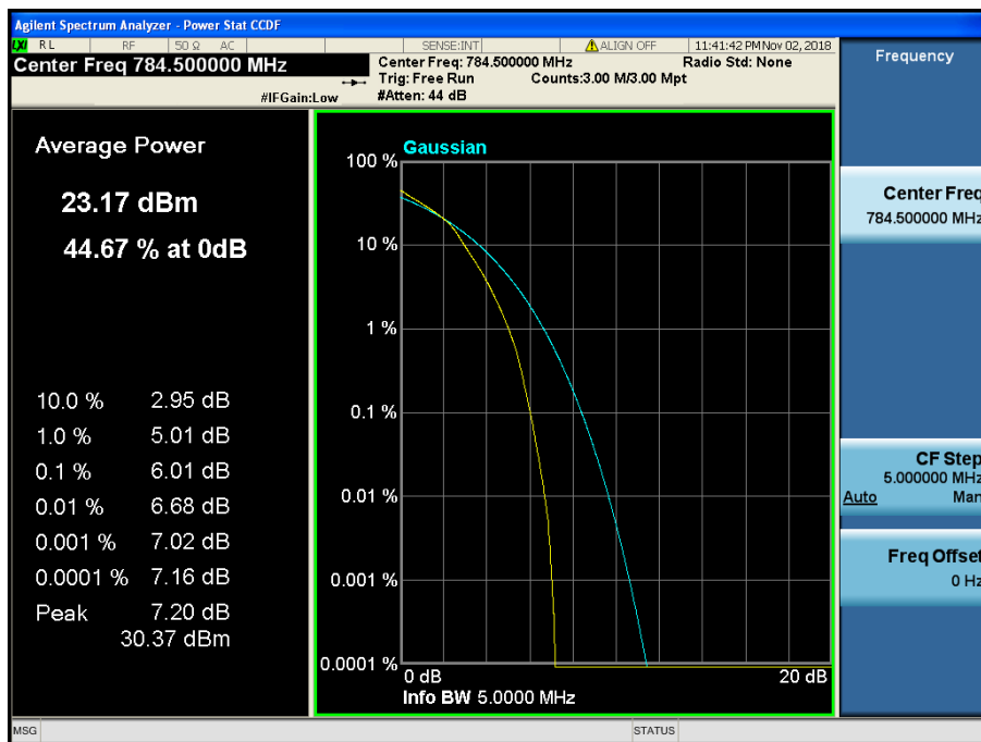
LTE Band 13 / 5 MHz / 16QAM - RB Size 25
