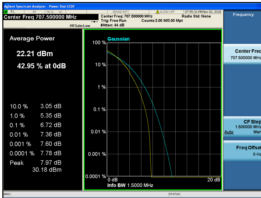
LTE Band 12 / 1.4 MHz / 64QAM - RB Size 6
