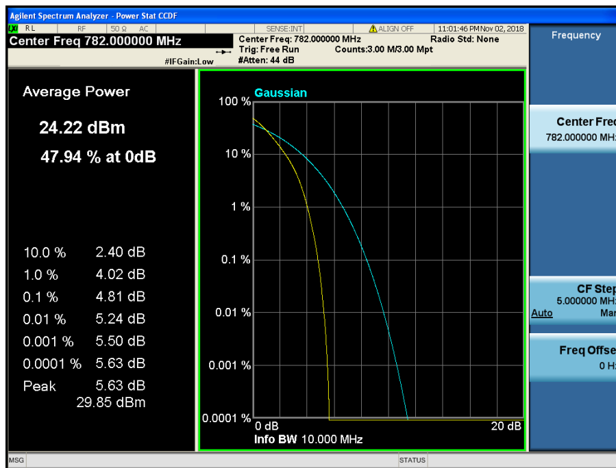
LTE Band 13 / 10 MHz / QPSK - RB Size 50
