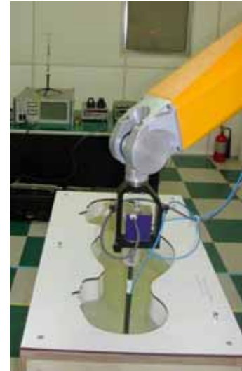
Figure 3. Photograph of the probe and the Phantom
