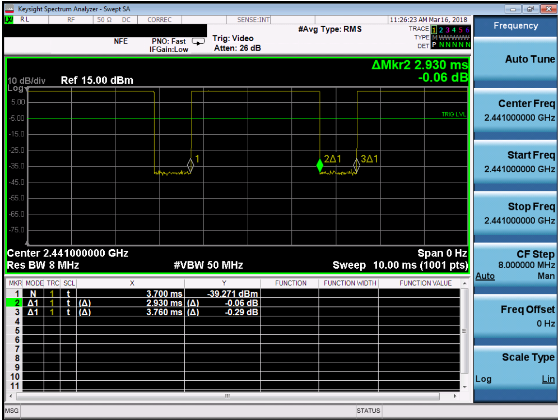
Figure 9-6 Bluetooth Transmission Plot
