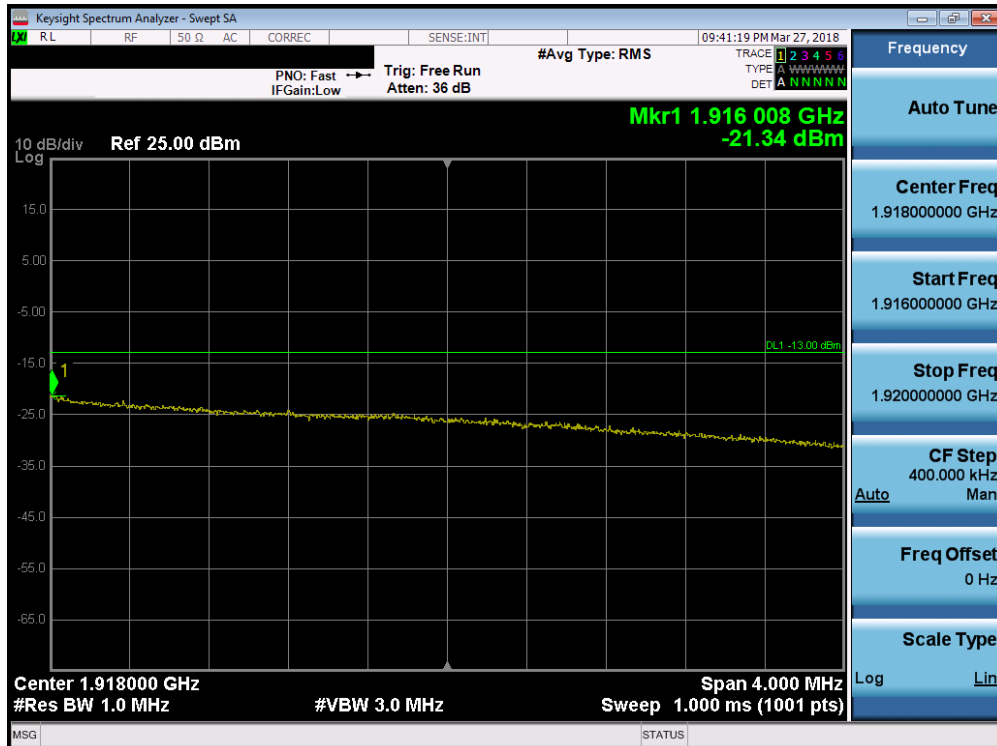
Plot 7-253. Upper Extended Band Edge Plot (Band 25 - 10.0MHz QPSK - Full RB Configuration)
