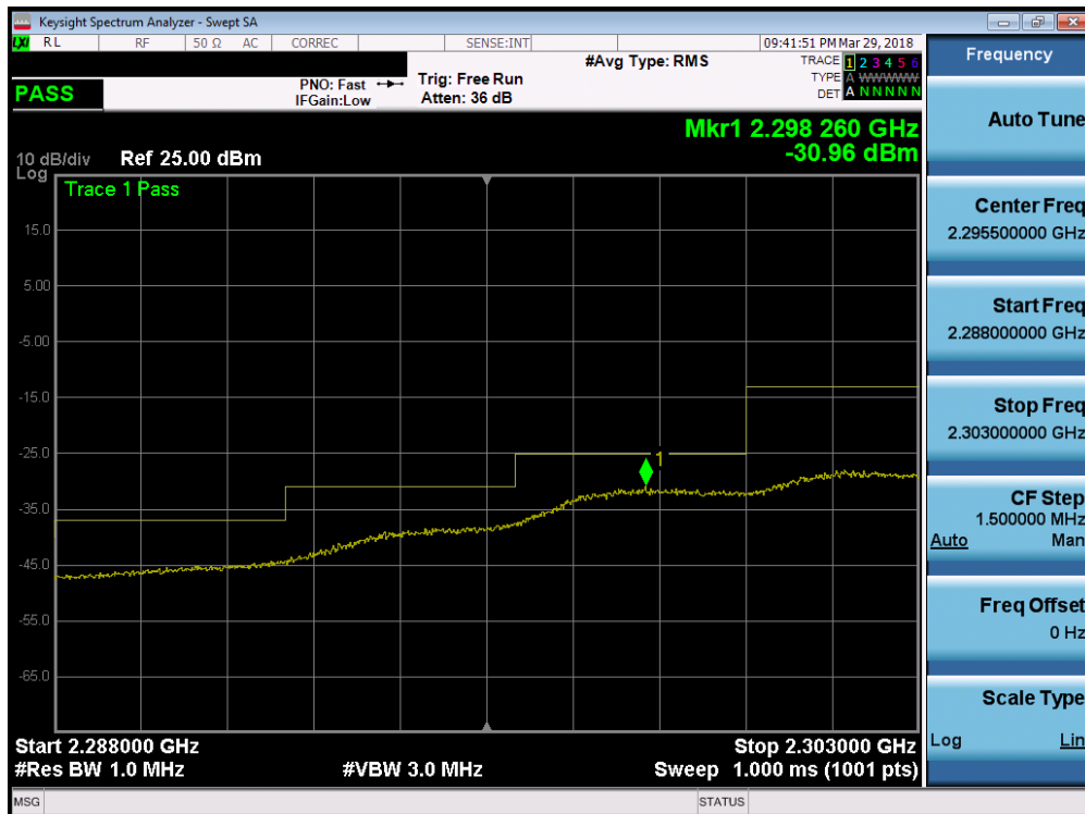
Plot 7-267. Lower Extended Band Edge Plot (Band 30 - 5.0MHz QPSK - Full RB Configuration)
