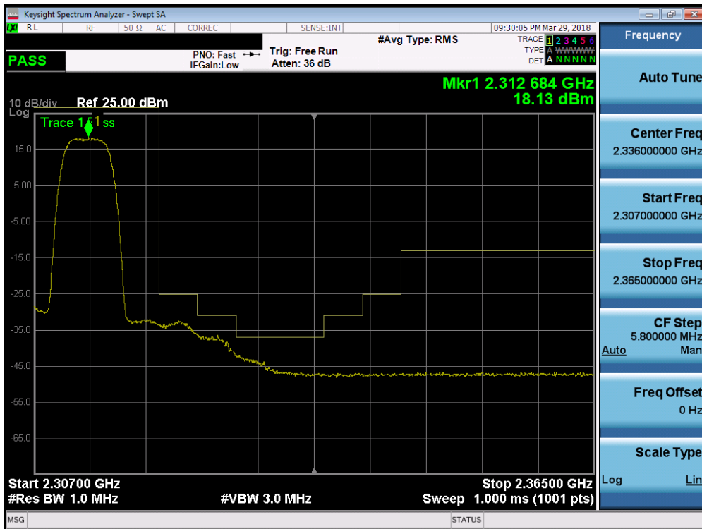
Plot 7-269. Upper Extended Band Edge Plot (Band 30 - 5.0MHz QPSK - Full RB Configuration)
