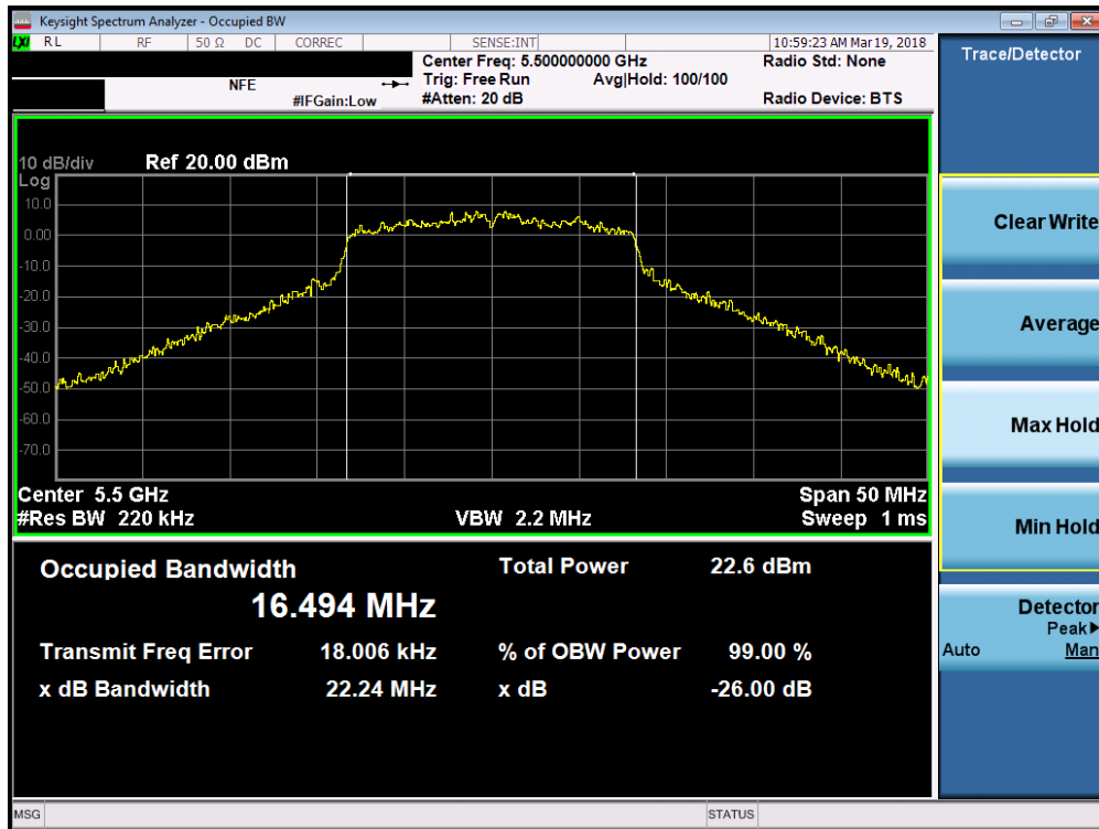
Plot 7-19. 26dB Bandwidth Plot SISO ANT1 (802.11a (UNII Band 2C) – Ch. 100)
