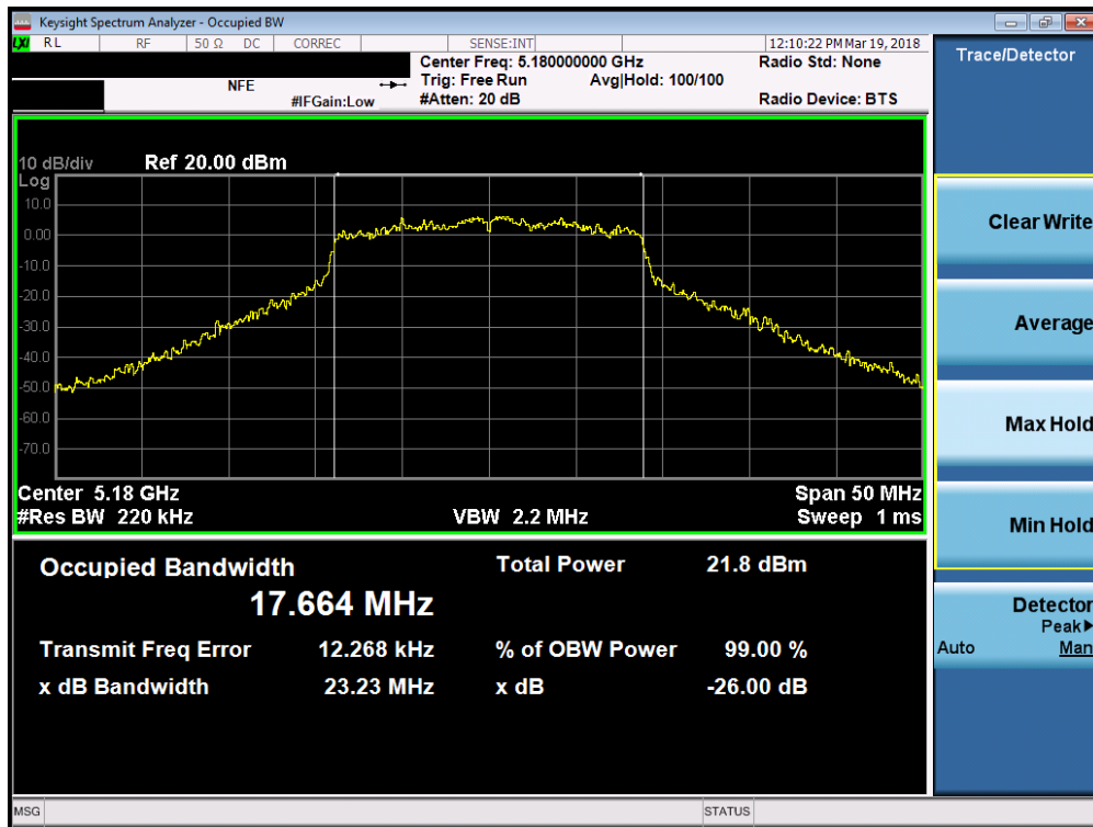
Plot 7-4. 26dB Bandwidth Plot SISO ANT1 (20MHz BW 802.11n (UNII Band 1) – Ch. 36)
