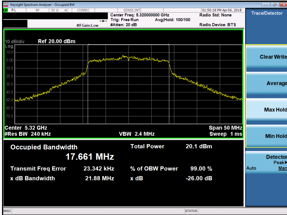
Plot 7-45. 26dB Bandwidth Plot SISO ANT2 (20MHz BW 802.11n (UNII Band 2A) – Ch. 64)
