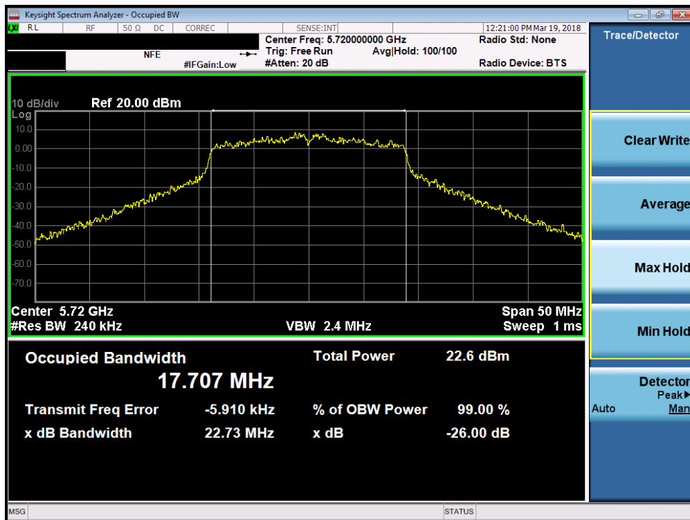
Plot 7-24. 26dB Bandwidth Plot SISO ANT1 (20MHz BW 802.11n (UNII Band 2C) – Ch. 144)
