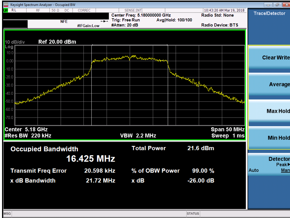
Plot 7-1. 26dB Bandwidth Plot SISO ANT1 (802.11a (UNII Band 1) – Ch. 36)
