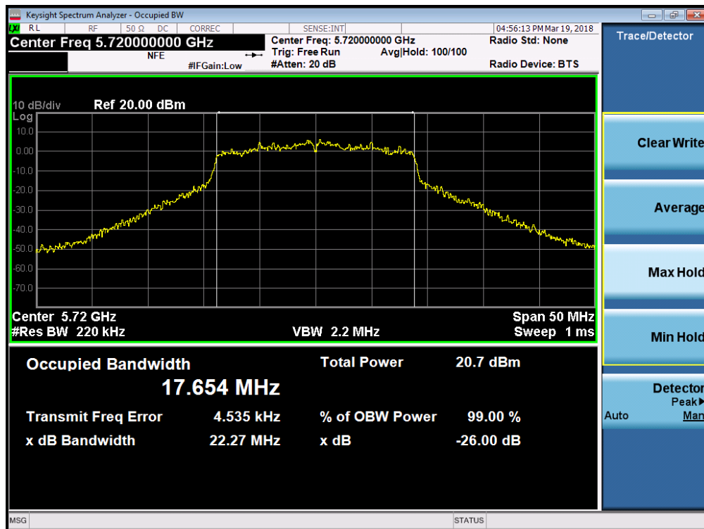
Plot 7-54. 26dB Bandwidth Plot SISO ANT2 (20MHz BW 802.11n (UNII Band 2C) – Ch. 144)
