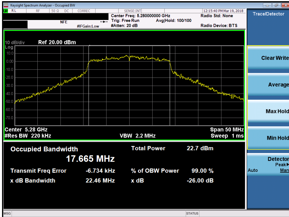
Plot 7-14. 26dB Bandwidth Plot SISO ANT1 (20MHz BW 802.11n (UNII Band 2A) – Ch. 56)
