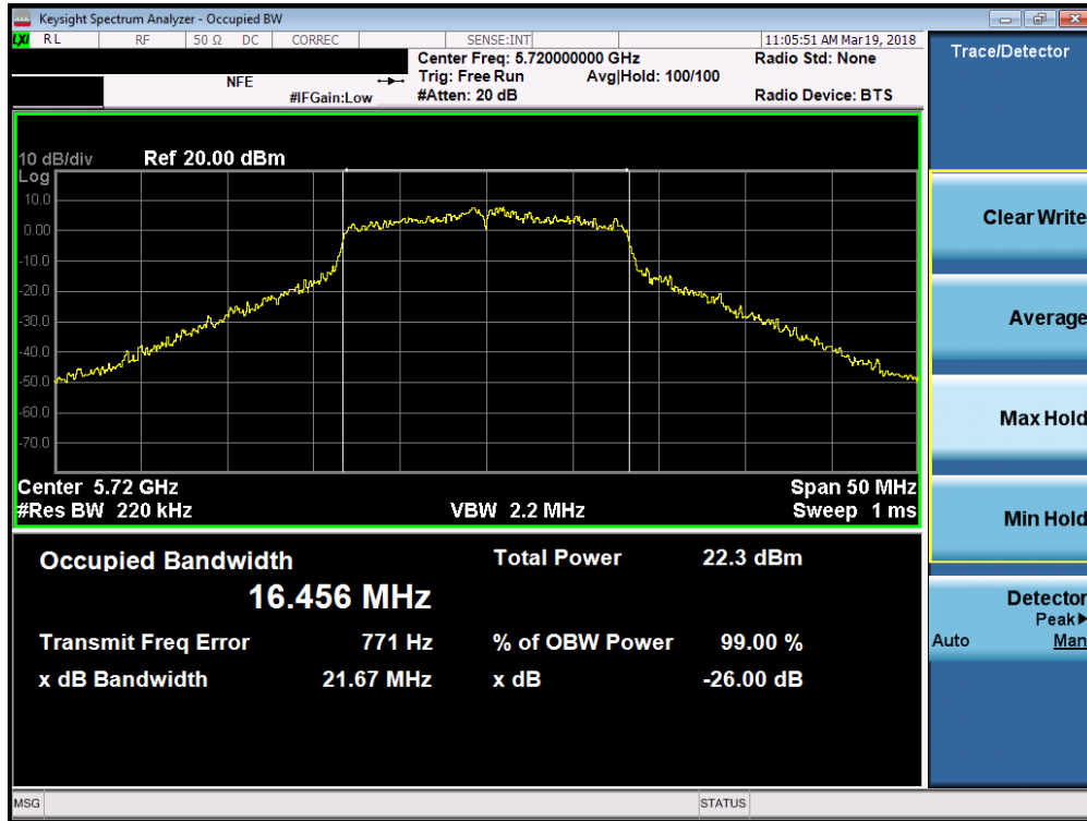
Plot 7-21. 26dB Bandwidth Plot SISO ANT1 (802.11a (UNII Band 2C) – Ch. 144)
