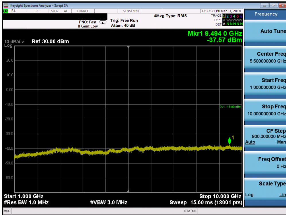
Plot 7-114. Conducted Spurious Plot (Band 26/5 - 10.0MHz QPSK - RB Size 1, RB Offset 0 - Low Channel)
