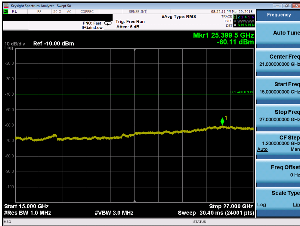
Plot 7-141. Conducted Spurious Plot (Band 30 - 5.0MHz QPSK - RB Size 1, RB Offset 0 - Low Channel)
