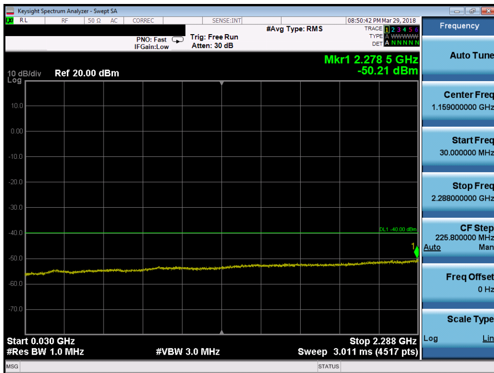
Plot 7-142. Conducted Spurious Plot (Band 30 - 5.0MHz QPSK - RB Size 1, RB Offset 0 - Mid Channel)
