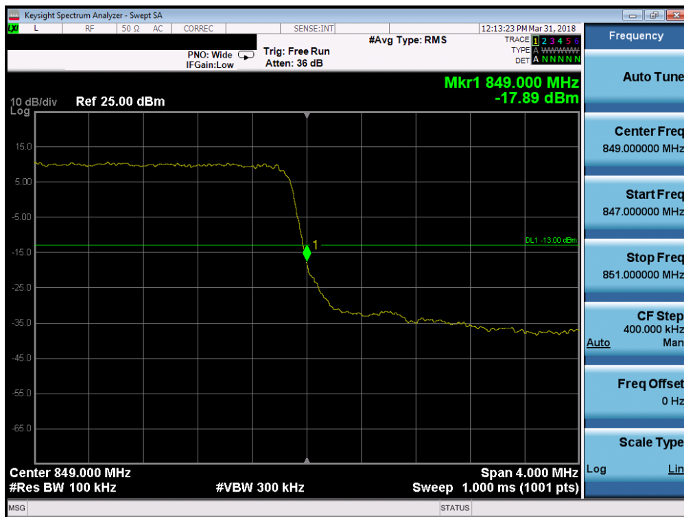
Plot 7-187. Lower Extended Band Edge Plot (Band 26/5 - 3.0MHz QPSK - Full RB Configuration)
