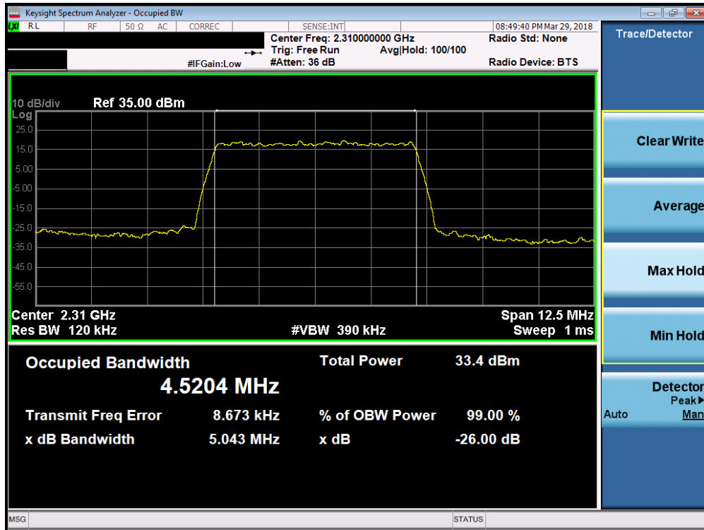
Plot 7-70. Occupied Bandwidth Plot (Band 30 - 5.0MHz QPSK - Full RB Configuration)
