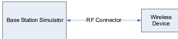
Figure 9-1 Power Measurement Setup
