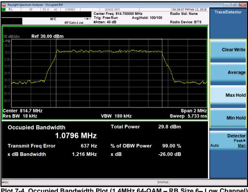
Plot 7-4. Occupied Bandwidth Plot (1.4MHz 64-QAM – RB Size 6– Low Channel)
