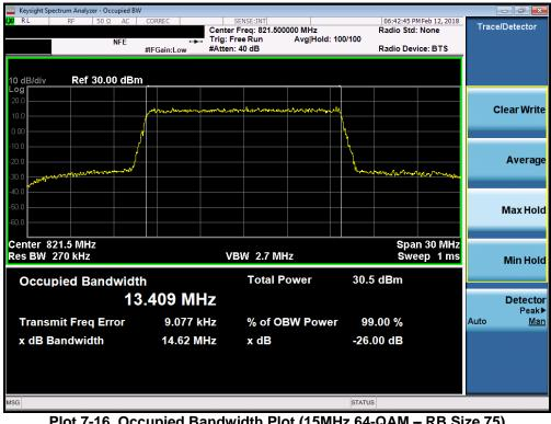
Plot 7-16. Occupied Bandwidth Plot (15MHz 64-QAM – RB Size 75)
