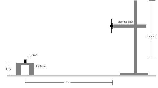
Figure 7-4. Radiated Test Setup <1GHz
