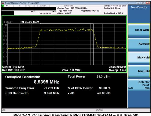
Plot 7-12. Occupied Bandwidth Plot (10MHz 16-QAM – RB Size 50)
