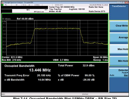
Plot 7-14. Occupied Bandwidth Plot (15MHz QPSK – RB Size 75)
