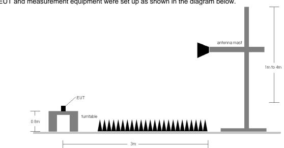
The EUT and measurement equipment were set up as shown in the diagram below.
