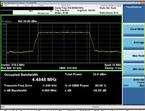
Plot 7-8. Occupied Bandwidth Plot (5MHz QPSK - RB Size 25- Low Channel)
