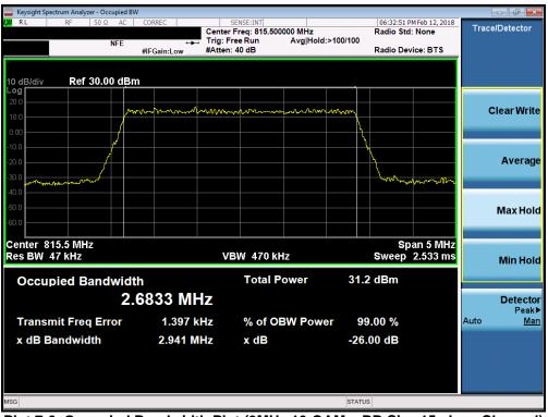
Plot 7-6. Occupied Bandwidth Plot (3MHz 16-QAM – RB Size 15– Low Channel)
