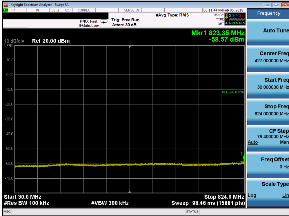
Plot 7-22. Conducted Spurious Plot (Band 26 - 10.0MHz QPSK - RB Size 1, RB Offset 0 - High Channel)
