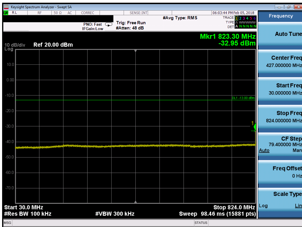
Plot 7-19. Conducted Spurious Plot (Band 26 - 10.0MHz QPSK - RB Size 1, RB Offset 0 - Mid Channel)
