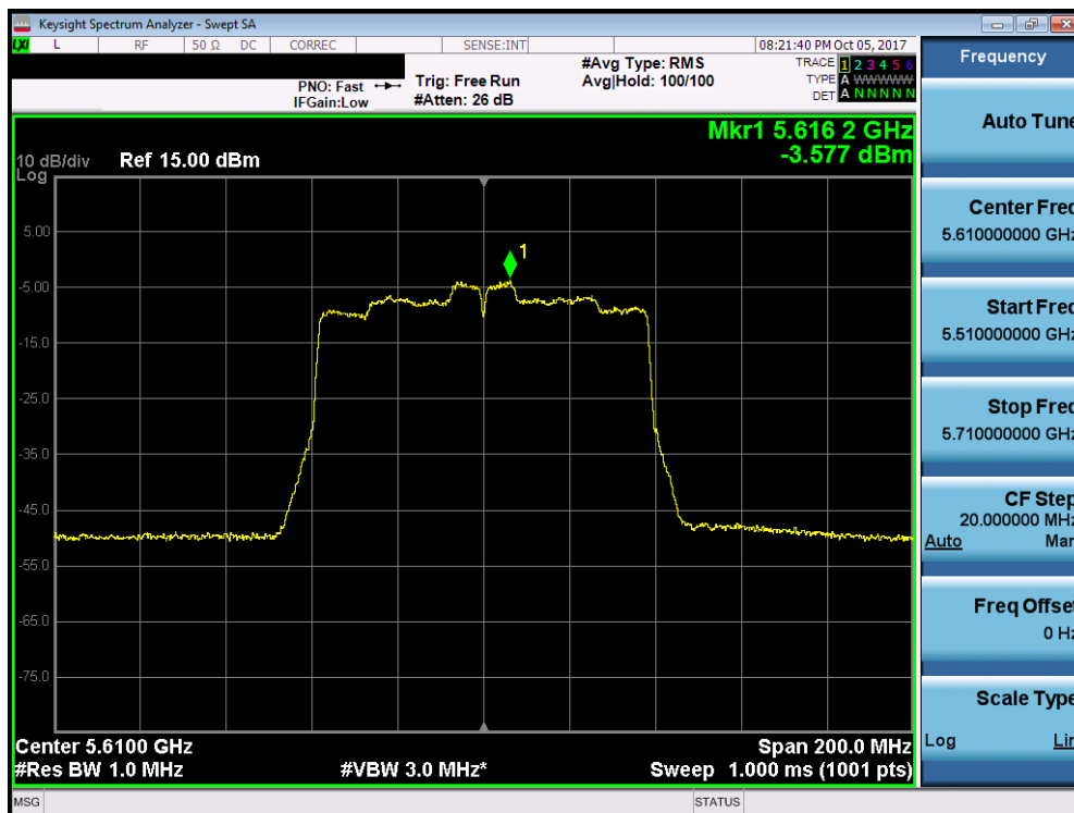
Plot 7-16. Power Spectral Density Plot (80MHz BW 802.11ac (UNII Band 2C) – Ch. 122)
