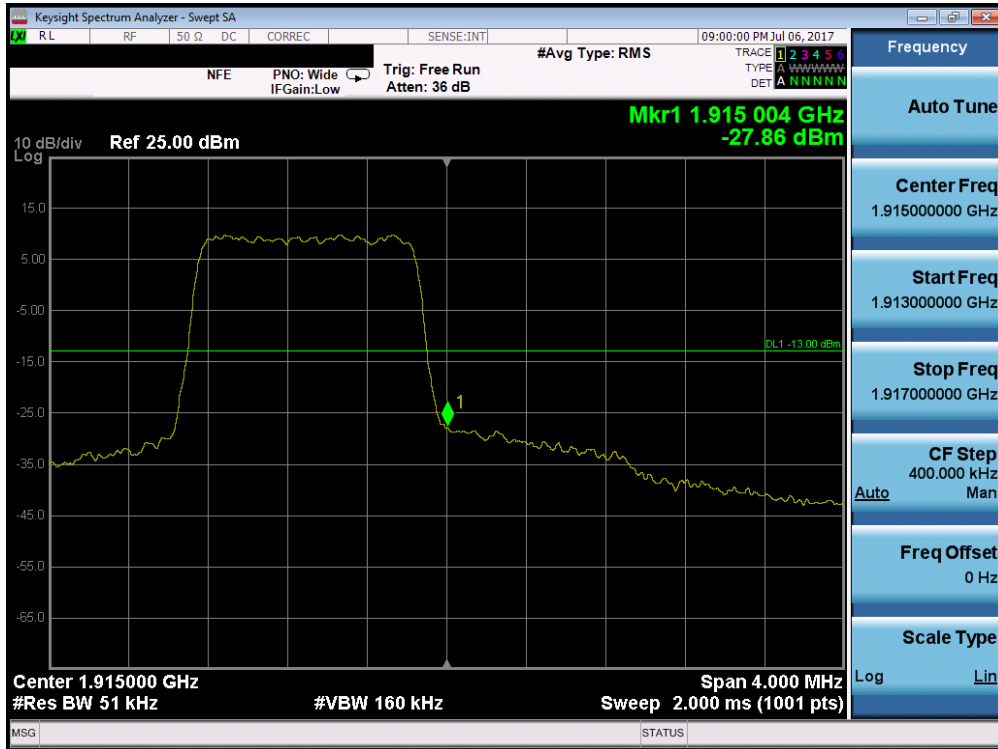
Plot 7-227. Upper Band Edge Plot (Band 25 – 1.4MHz QPSK – RB Size 6)
