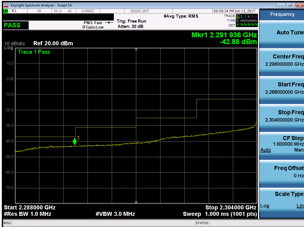
Plot 7-260. Lower Extended Band Edge Plot (Band 30 – 10.0MHz QPSK – RB Size 50)
