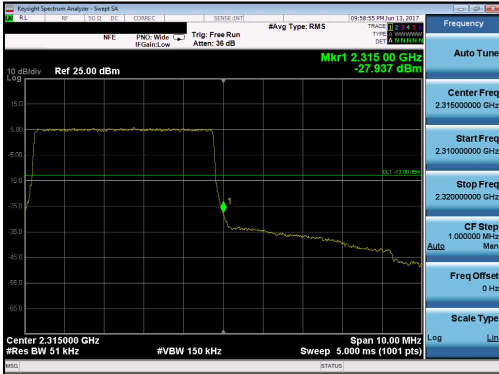
Plot 7-257. Upper Band Edge Plot (Band 30 – 5.0MHz QPSK – RB Size 25)
