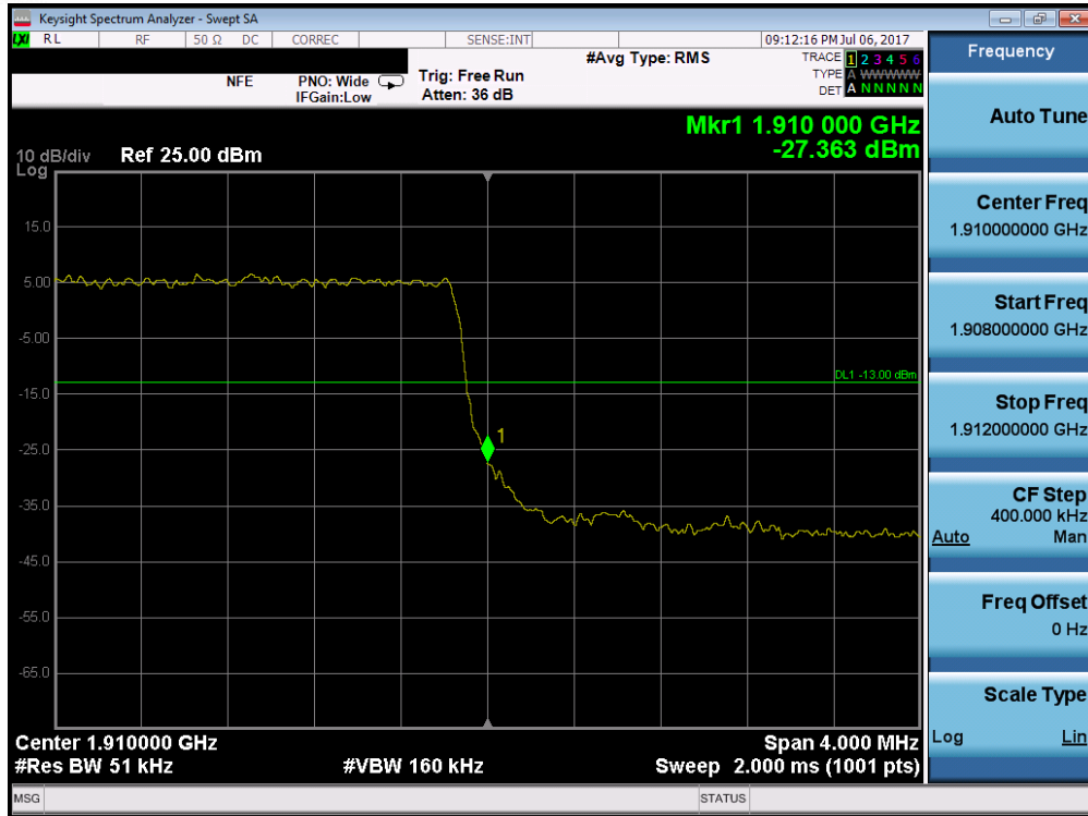
Plot 7-235. Upper Band Edge Plot (Band 2 – 3.0MHz QPSK – RB Size 15)
