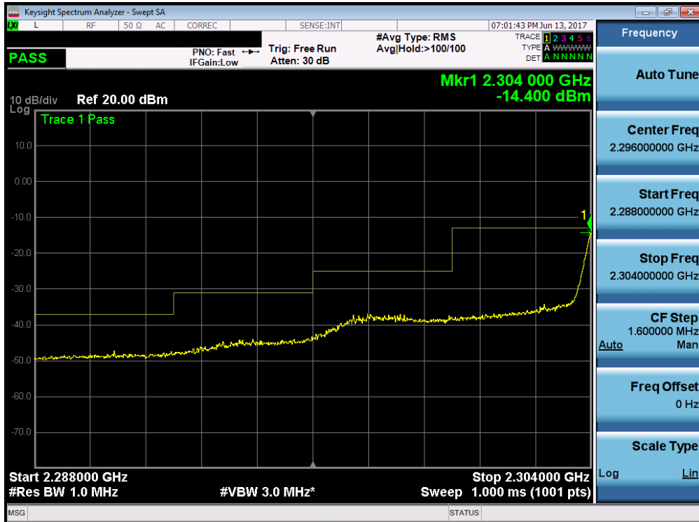
Plot 7-256. Lower Extended Band Edge Plot (Band 30 – 5.0MHz QPSK – RB Size 25)
