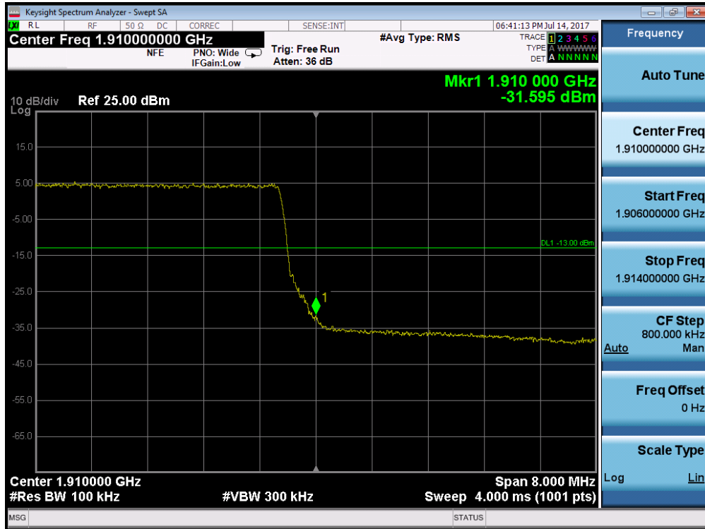
Plot 7-245. Upper Band Edge Plot (Band 2 – 10.0MHz QPSK – RB Size 50)
