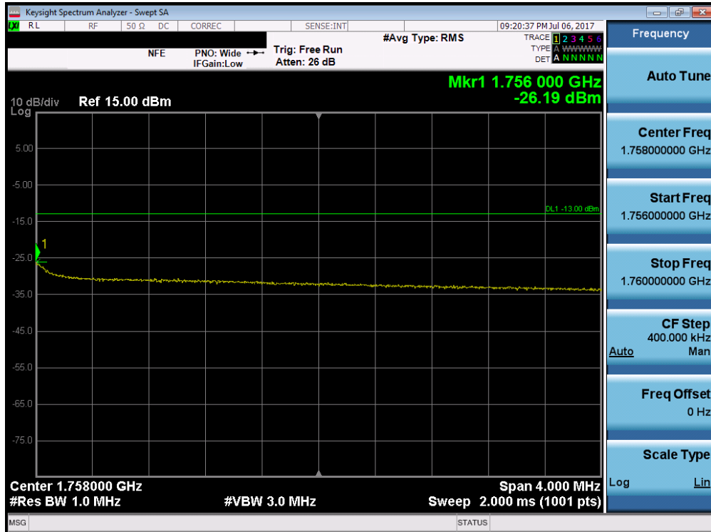
Plot 7-212. Upper Extended Band Edge Plot (Band 4 – 10.0MHz QPSK – RB Size 50)
