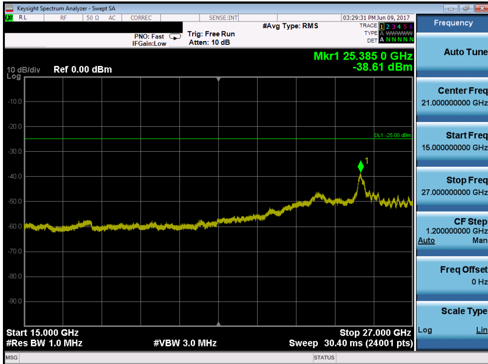
Plot 7-150. Conducted Spurious Plot (Band 7 – 10.0MHz QPSK – RB Size 1, RB Offset 0 – Mid Channel)
