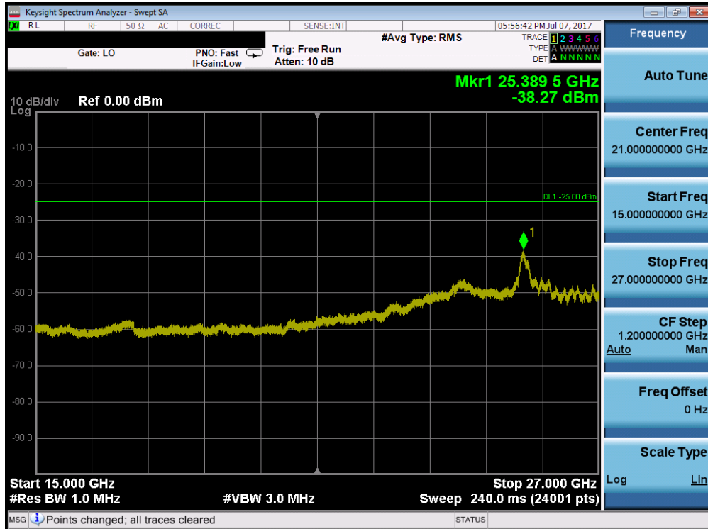
Plot 7-156. Conducted Spurious Plot (Band 41 – 10.0MHz QPSK – RB Size 1, RB Offset 0 – Low Channel)
