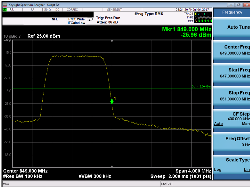
Plot 7-182. Upper Band Edge Plot (Band 5 – 1.4MHz QPSK – RB Size 6)
