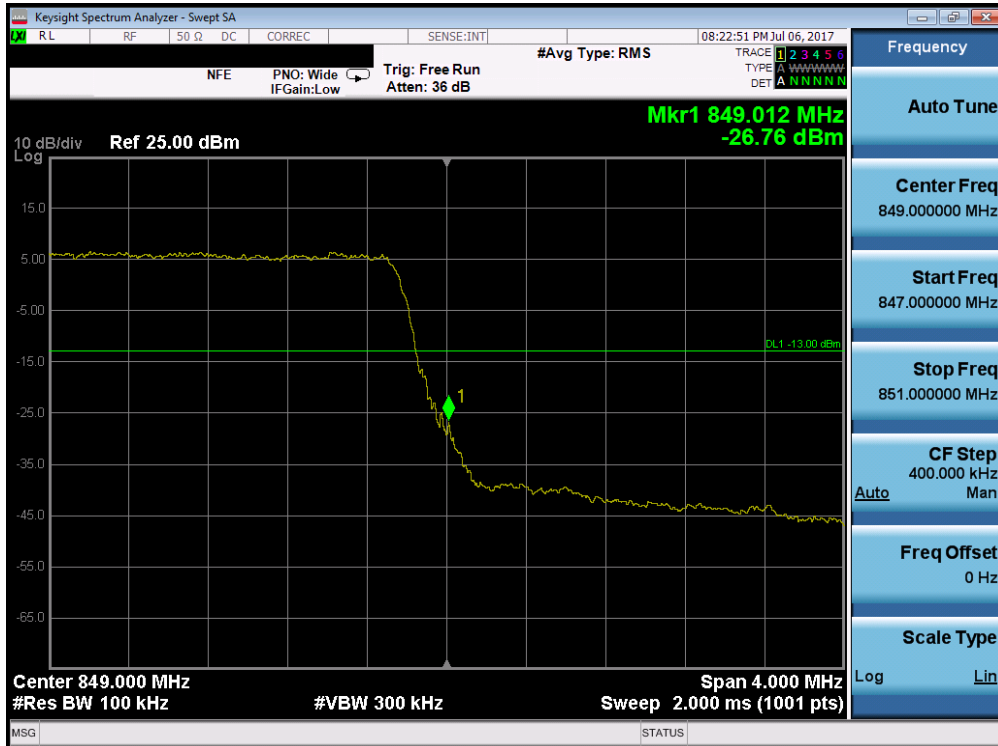
Plot 7-186. Upper Band Edge Plot (Band 5 – 5.0MHz QPSK – RB Size 25)
