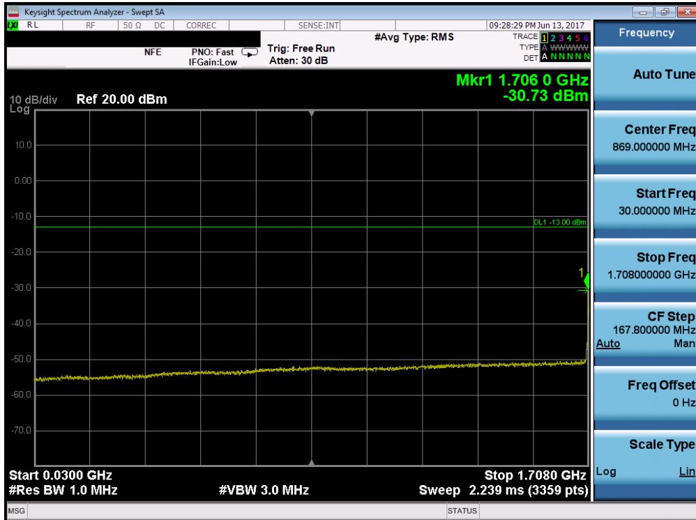
Plot 7-118. Conducted Spurious Plot (Band 4/66 – 5.0MHz QPSK – RB Size 1, RB Offset 0 – Low Channel)
