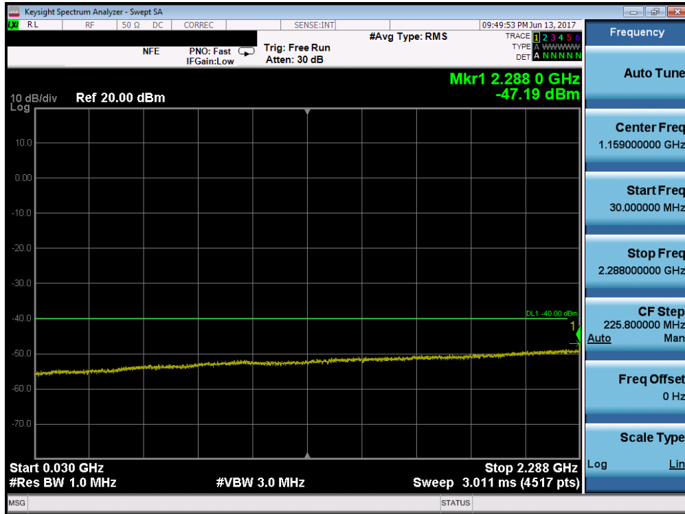
Plot 7-139. Conducted Spurious Plot (Band 30 – 5.0MHz QPSK – RB Size 1, RB Offset 0 – Mid Channel)
