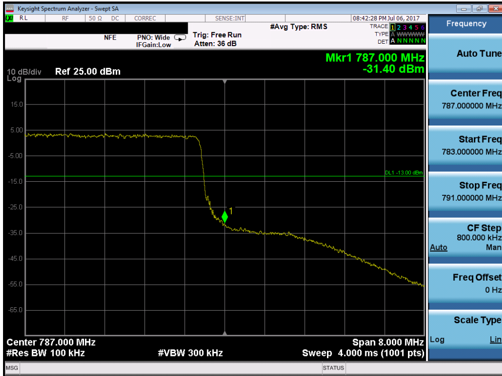
Plot 7-179. Upper Band Edge Plot (Band 13 – 10.0MHz QPSK – RB Size 50)
