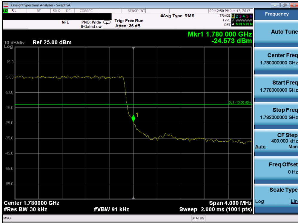
Plot 7-197. Upper Band Edge Plot (Band 66 – 3.0MHz QPSK – RB Size 15)
