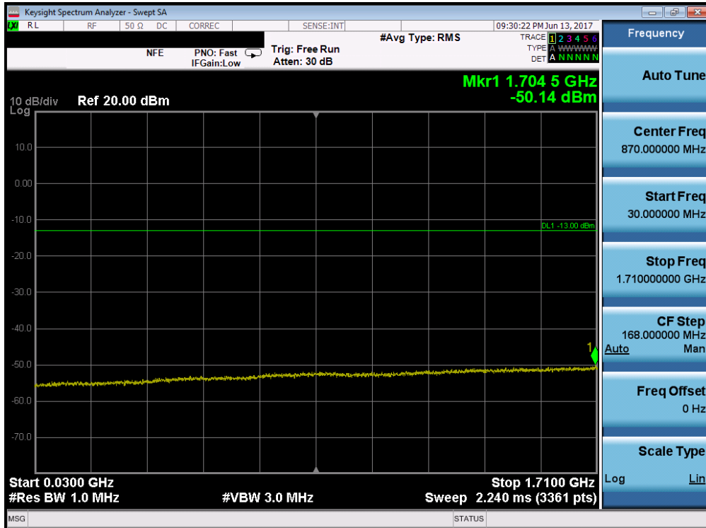
Plot 7-124. Conducted Spurious Plot (Band 4/66 – 5.0MHz QPSK – RB Size 1, RB Offset 0 – High Channel)
