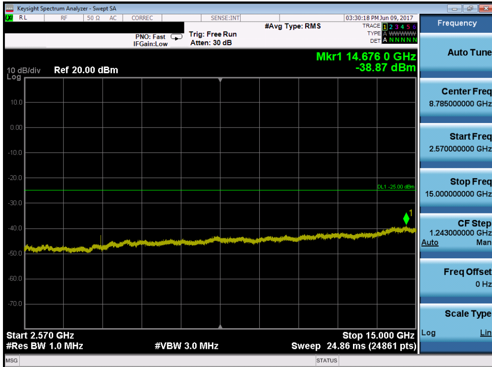
Plot 7-146. Conducted Spurious Plot (Band 7 – 10.0MHz QPSK – RB Size 1, RB Offset 0 – Low Channel)
