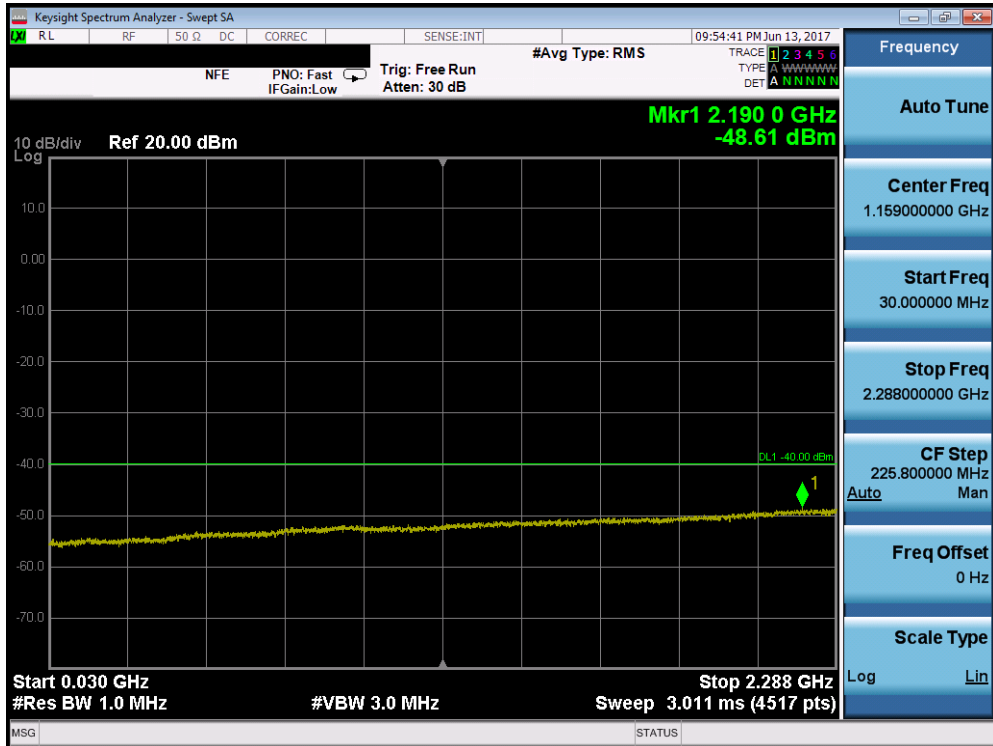
Plot 7-136. Conducted Spurious Plot (Band 30 – 5.0MHz QPSK – RB Size 1, RB Offset 0 – Low Channel)
