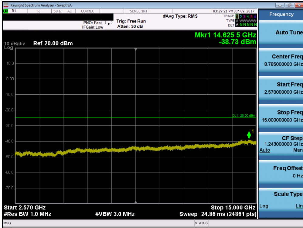
Plot 7-149. Conducted Spurious Plot (Band 7 – 10.0MHz QPSK – RB Size 1, RB Offset 0 – Mid Channel)
