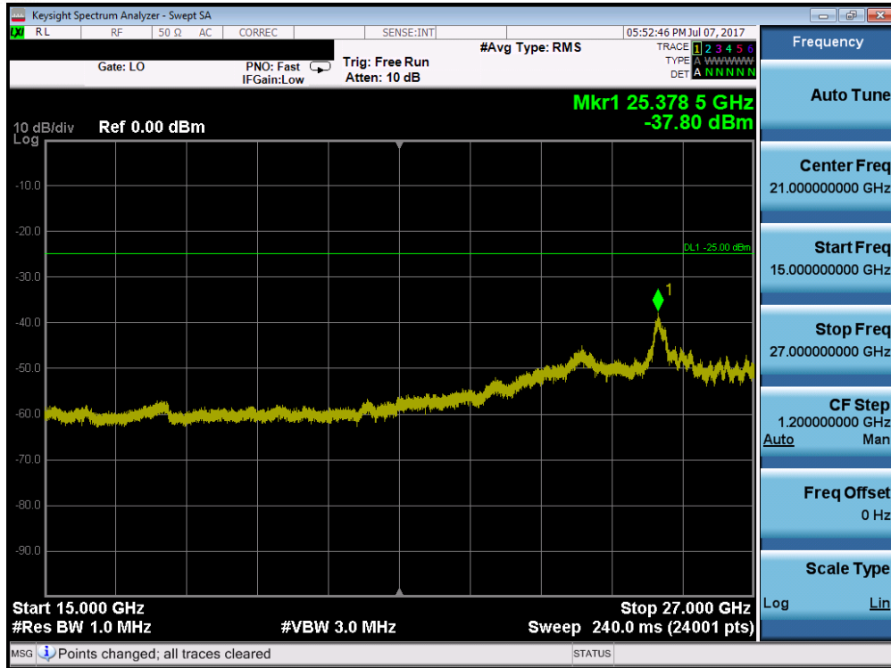
Plot 7-159. Conducted Spurious Plot (Band 41 – 10.0MHz QPSK – RB Size 1, RB Offset 0 – Mid Channel)
