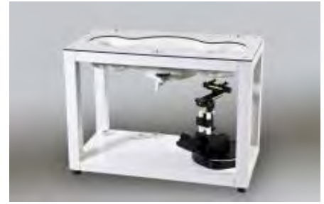
Figure 3.6 SAM Twin Phantom
