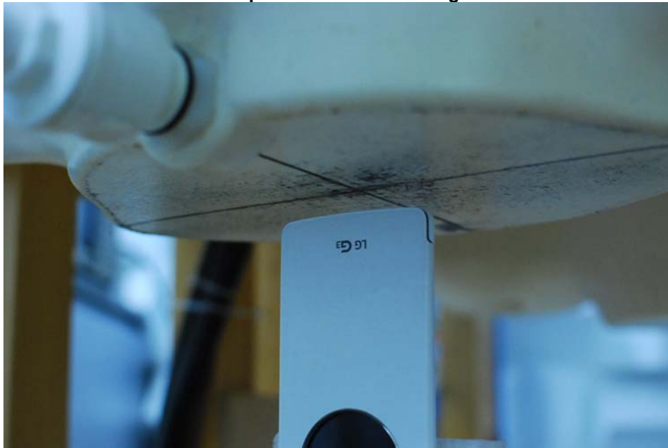
SAR Test Setup Photo 16: Bottom Edge with Wireless Charging Cover Closed at 1.0 cm
