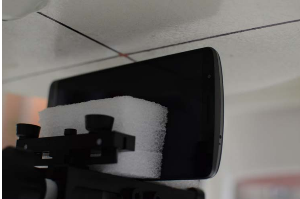
SAR Test Setup Photo 19: Left Edge at 1.0 cm
