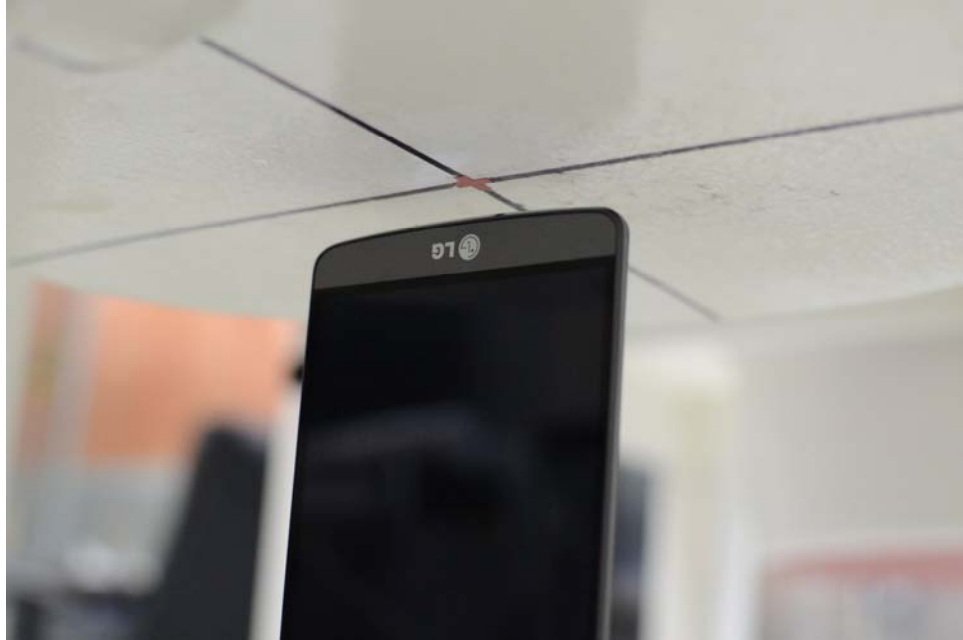
SAR Test Setup Photo 15: Bottom Edge at 1.0 cm
