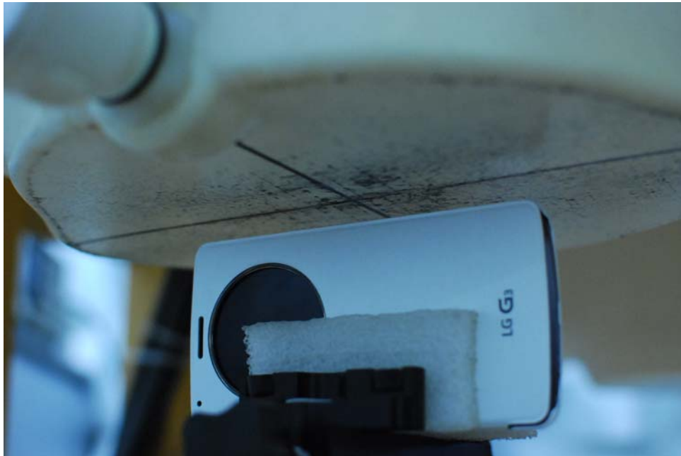
SAR Test Setup Photo 18: Right Edge with Wireless Charging Cover Closed at 1.0 cm
