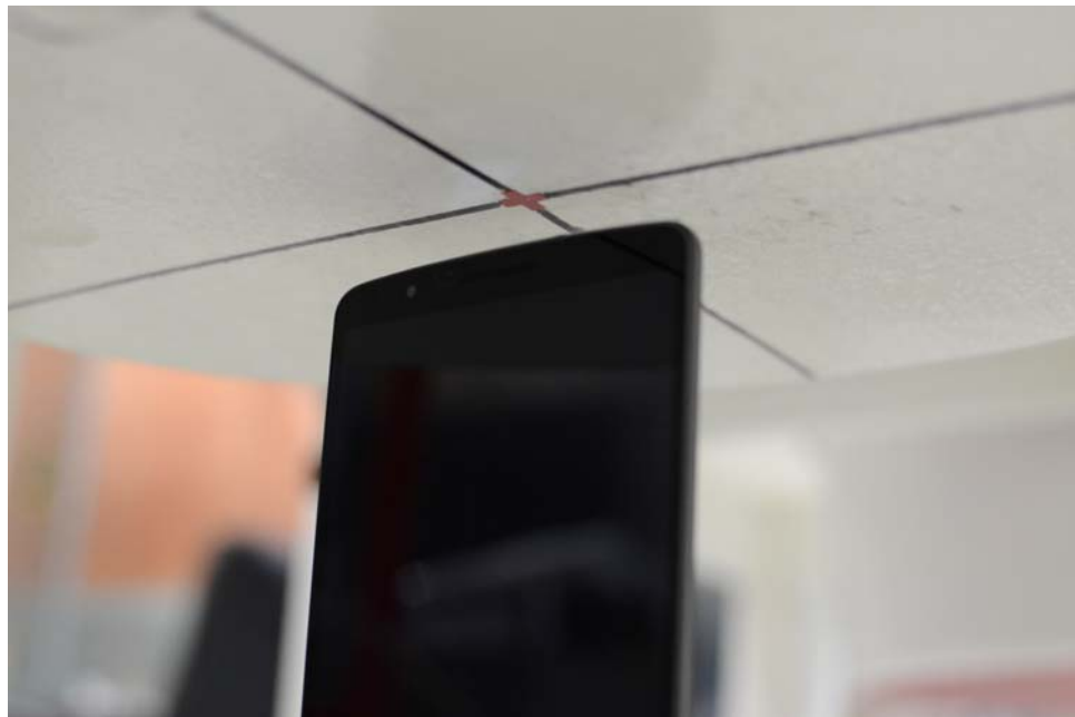
SAR Test Setup Photo 14: Top Edge at 1.0 cm
