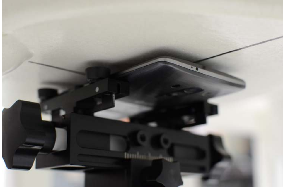
SAR Test Setup Photo 13: Front Side at 1.0 cm
