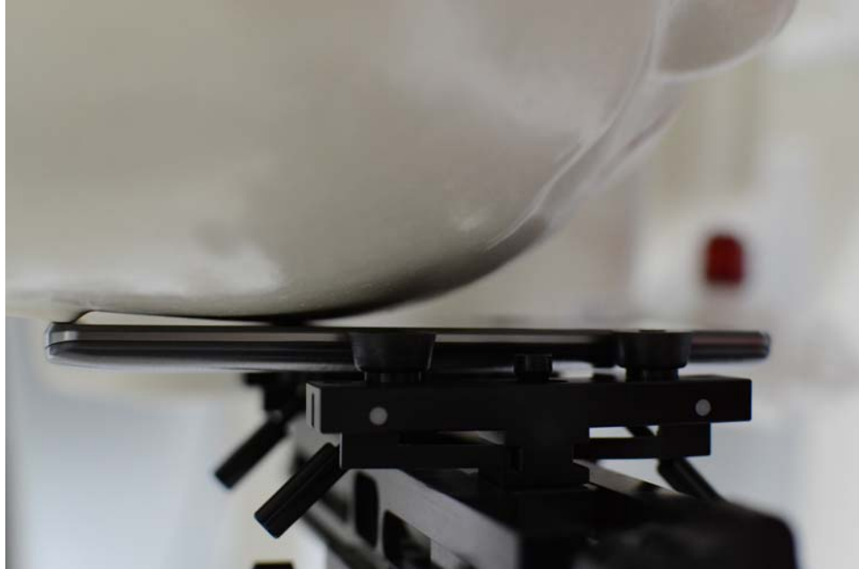
SAR Test Setup Photo 1: Right Cheek
