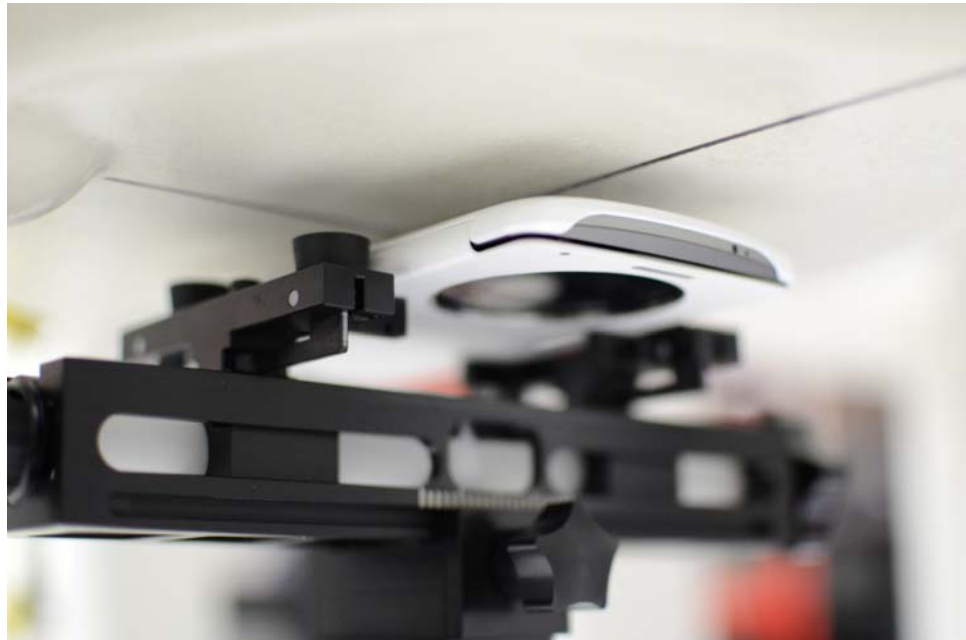
SAR Test Setup Photo 12: Back Side with Wireless Charging Cover Closed at 1.0 cm
