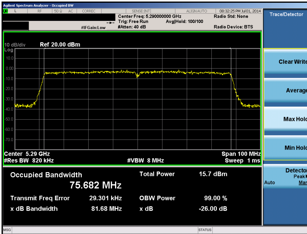
Plot 6-18. 26dB Bandwidth Plot (80MHz BW 802.11ac (UNII Band 2A) – Ch. 58)
