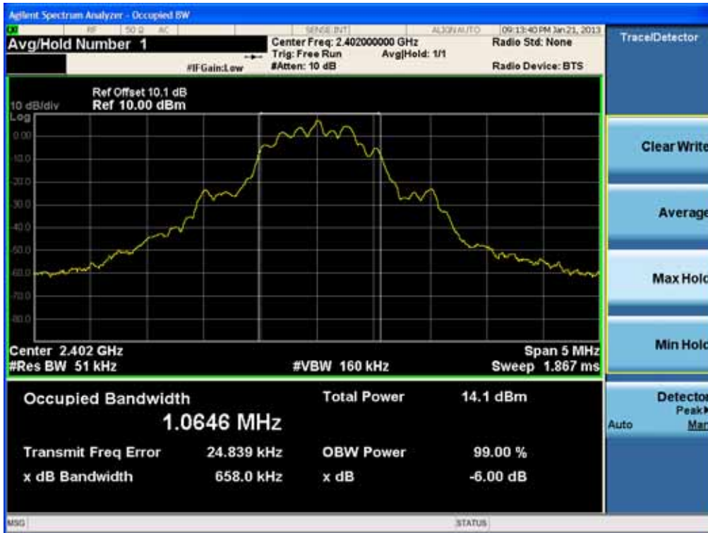
6dB Bandwidth plot (Low-CH 0)
