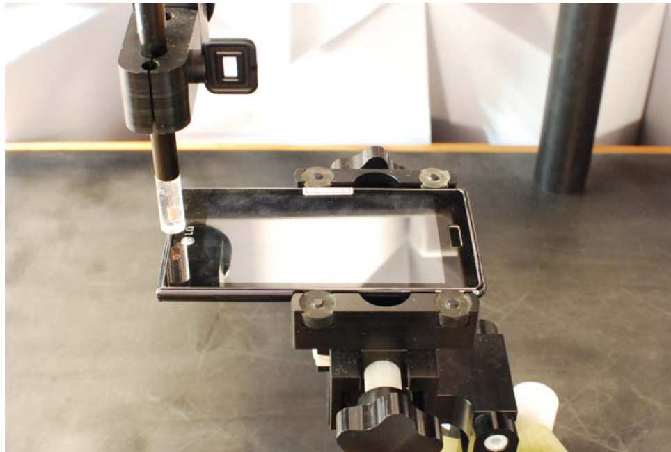
Figure 13-1 Test Setup for Wireless Device
