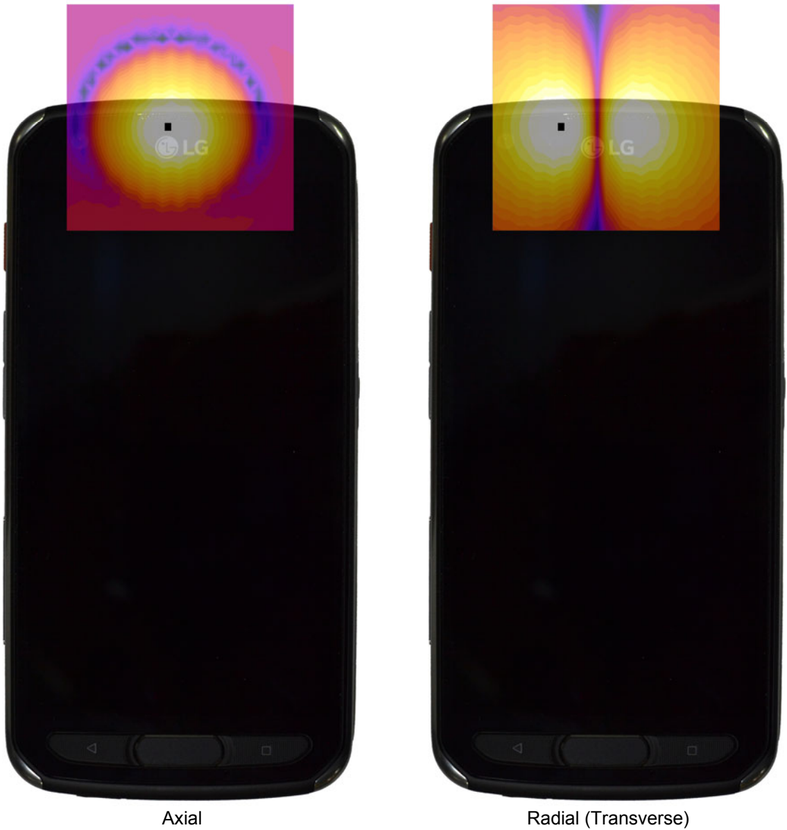
Figure 13-3 T-Coil Scan Overlay Magnetic Field Distributions
