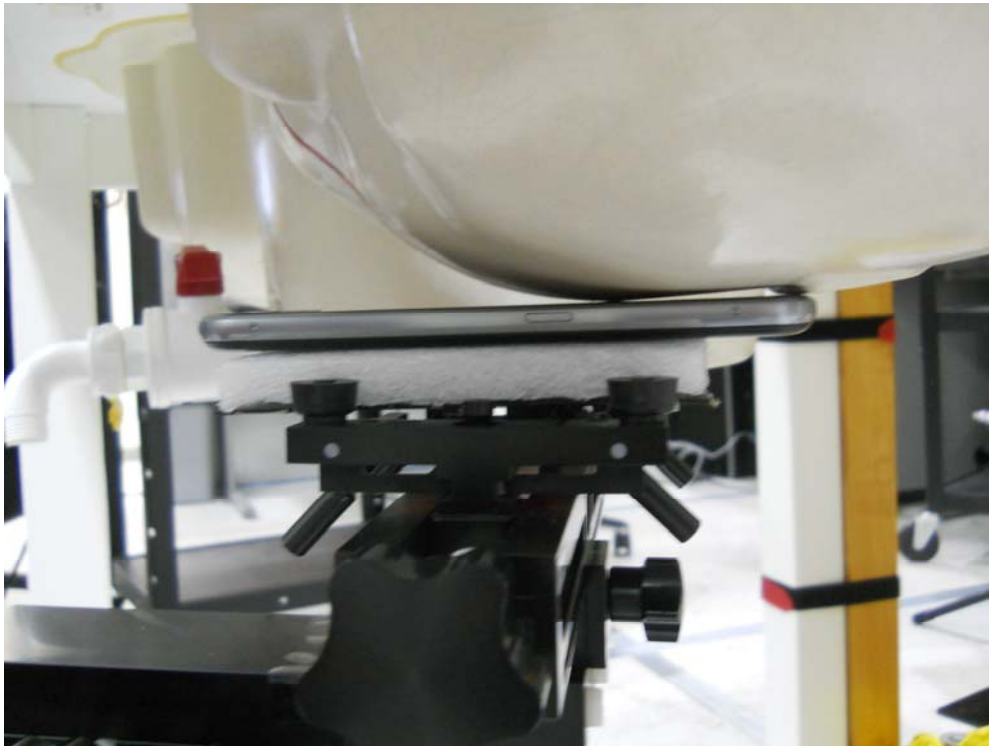
SAR Test Setup Photo 3: Left Cheek
