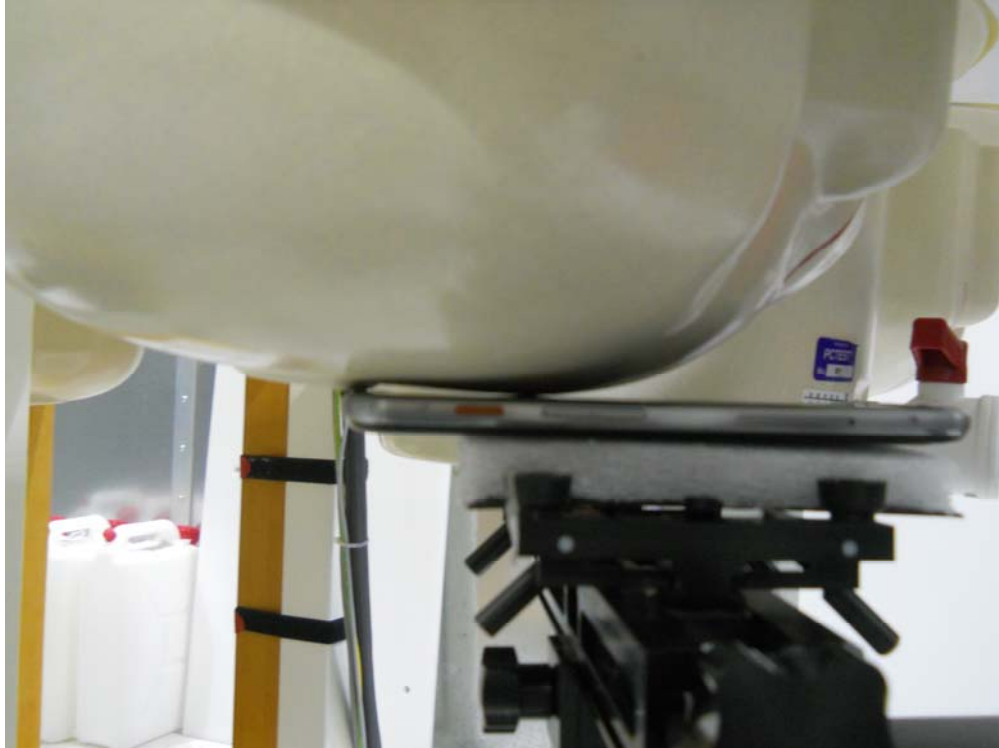
SAR Test Setup Photo 1: Right Cheek
