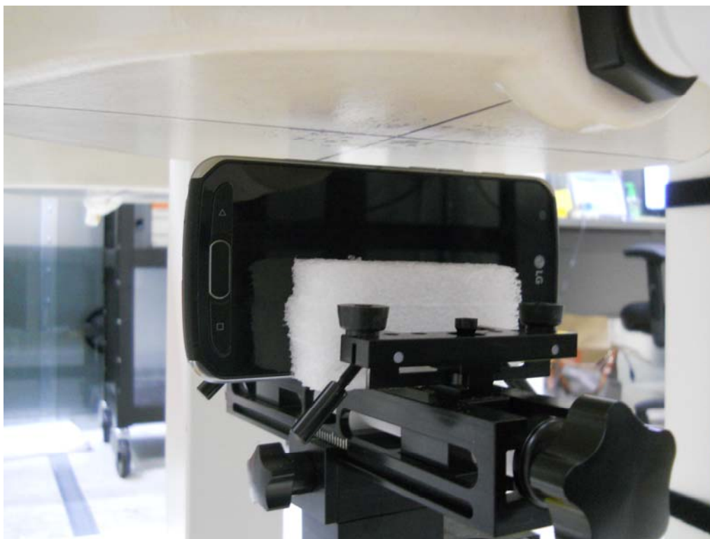
SAR Test Setup Photo 11: Left Edge at 1.0 cm
