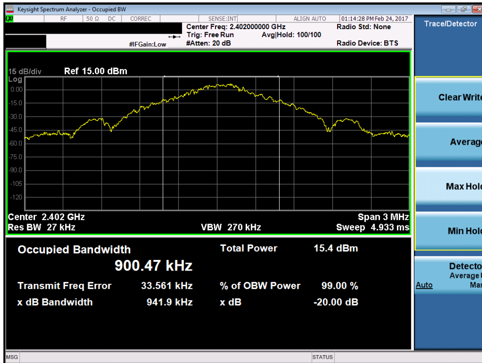
Plot 7-1. 20dB Bandwidth Plot (Bluetooth, 1Mbps – Ch. 0)
