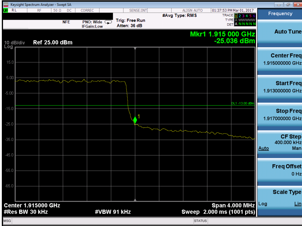
Plot 7-145. Upper Band Edge Plot (Band 25 – 3.0MHz QPSK – RB Size 15)
