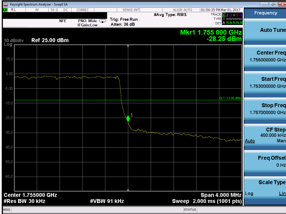
Plot 7-121. Upper Band Edge Plot (Band 4 – 3.0MHz QPSK – RB Size 15)
