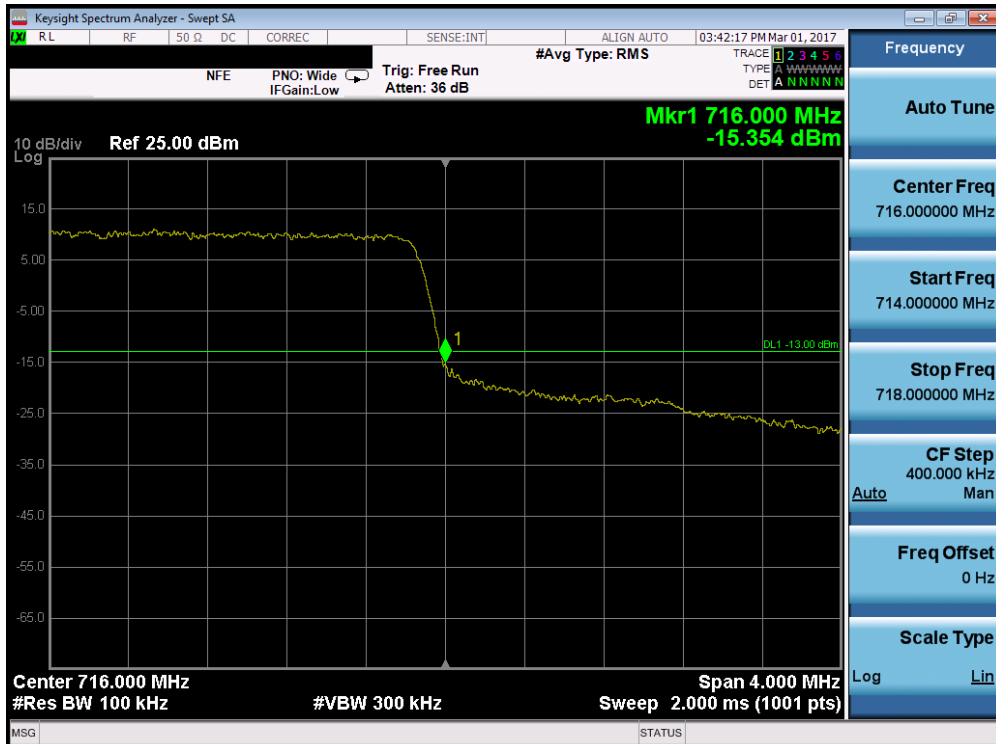
Plot 7-94. Upper Band Edge Plot (Band 12 – 3.0MHz QPSK – RB Size 15)
