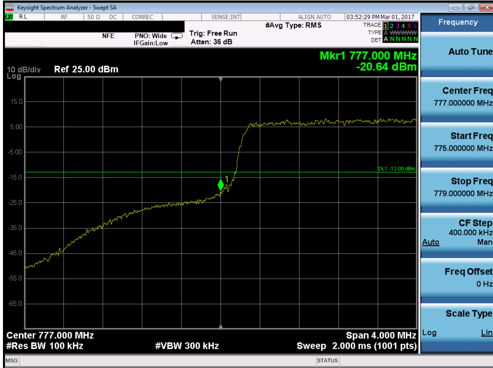
Plot 7-99. Lower Band Edge Plot (Band 13 – 5.0MHz QPSK – RB Size 25)
