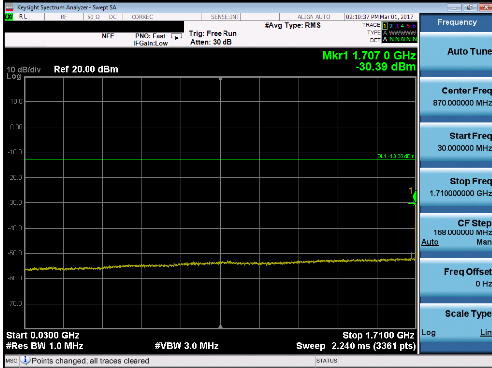
Plot 7-75. Conducted Spurious Plot (Band 4 – 20.0MHz QPSK – RB Size 1, RB Offset 0 – Mid Channel)
