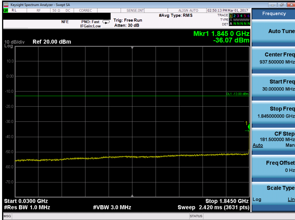
Plot 7-64. Conducted Spurious Plot (PCS WCDMA Mode – Ch. 9262)
