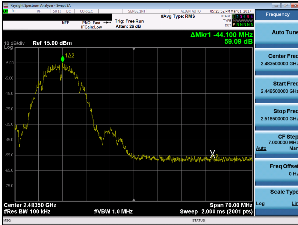
Plot 7-20. Band Edge Plot (802.11b – Ch. 11)
