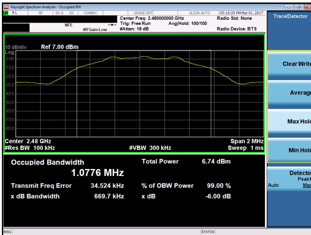
Plot 7-3. 6dB Bandwidth Plot (Bluetooth (LE) – Ch. 39)
