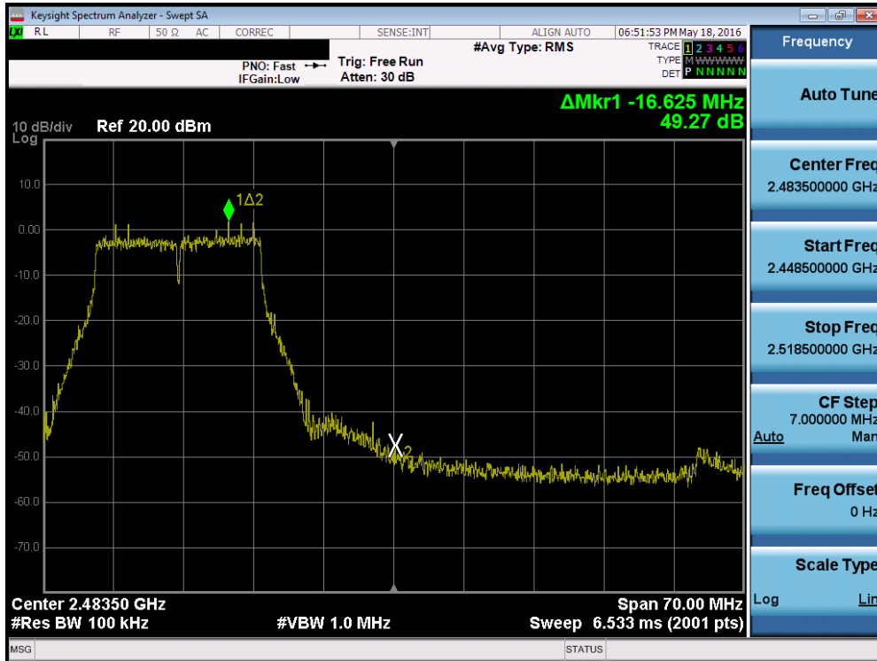
Plot 7-26. Band Edge Plot (802.11g – Ch. 11)
