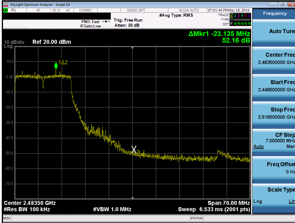
Plot 7-25. Band Edge Plot (802.11g – Ch. 10)
