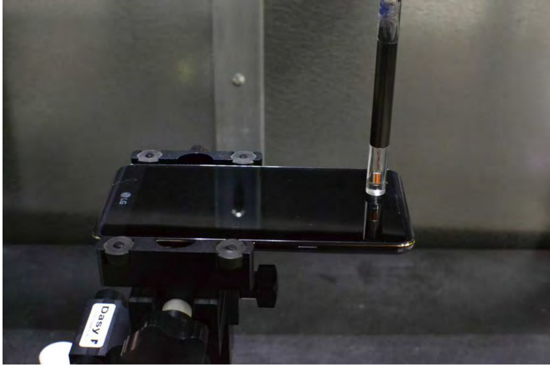
Figure 13-1 Test Setup for Wireless Device
