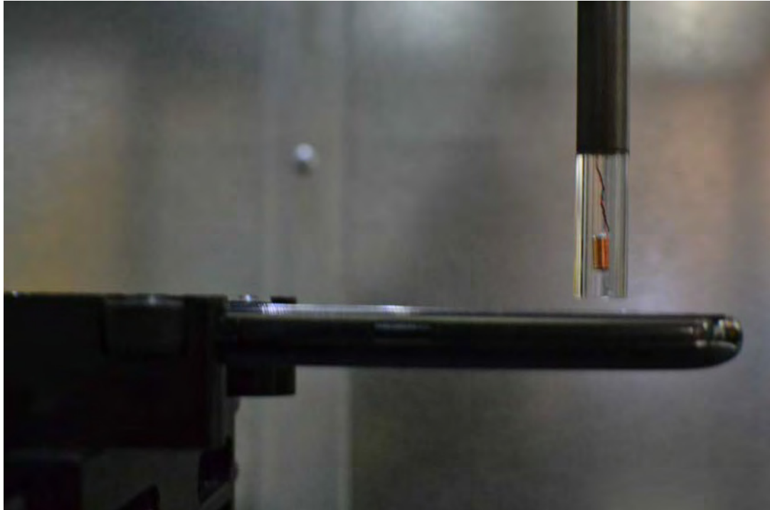
Figure 13-2 Test Setup for Wireless Device
