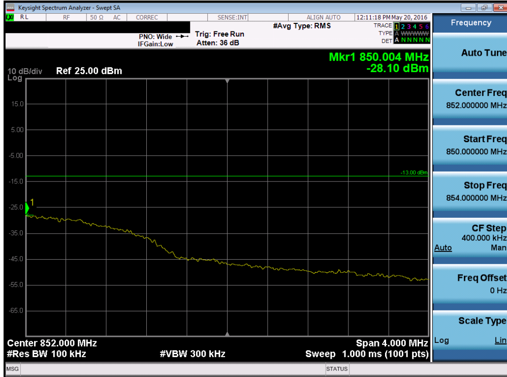
Plot 7-124. Upper Extended Band Edge Plot (Band 5 – Band 5 – 3.0MHz QPSK – RB Size 15)
