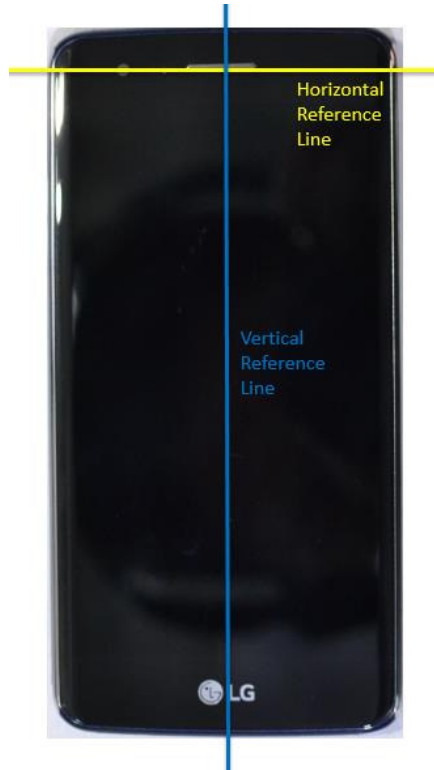
SAR Test Setup Photo 11 – Horizontal and Vertical Reference Lines
