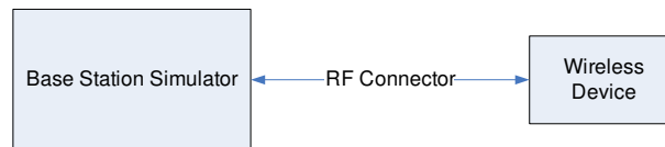
Figure 9-1 Power Measurement Setup
