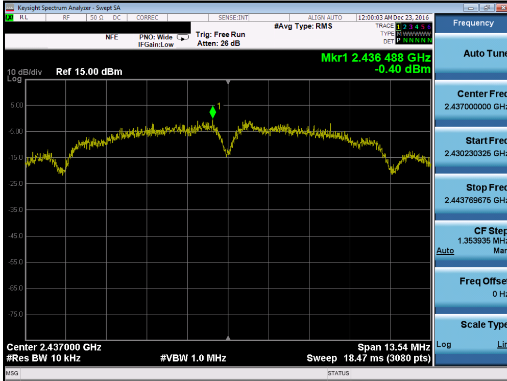
Plot 7-11. Power Spectral Density Plot (802.11b – Ch. 6)
