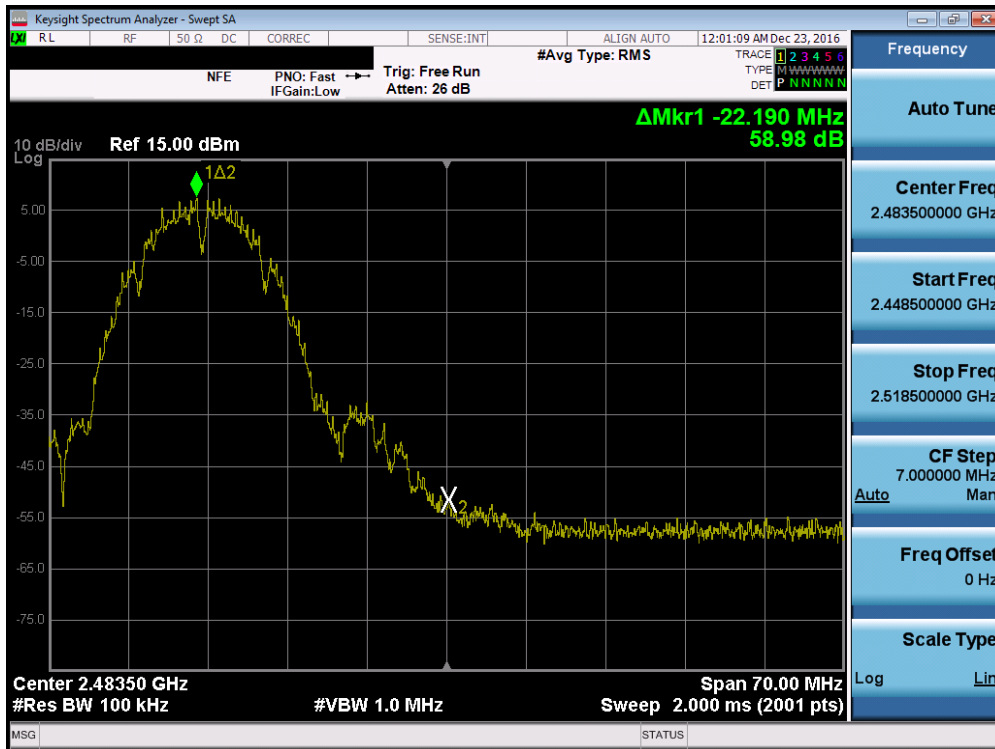
Plot 7-20. Band Edge Plot (802.11b – Ch. 11)
