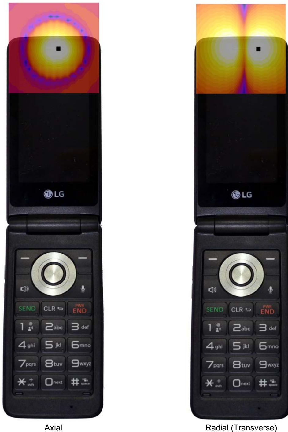
Axial Radial (Transverse) Figure 13-3 T-Coil Scan Overlay Magnetic Field Distributions
