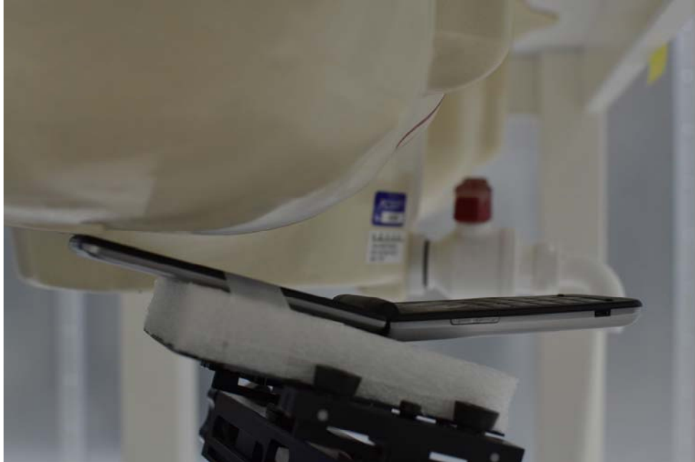
SAR Test Setup Photo 3 Right Tilt
