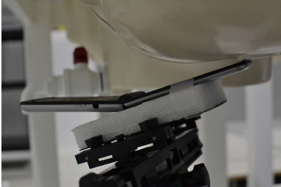
SAR Test Setup Photo 7 Left Tilt
