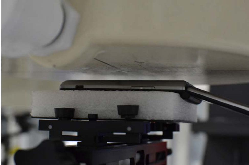
SAR Test Setup Photo 9 Back Side Open at 10 mm
