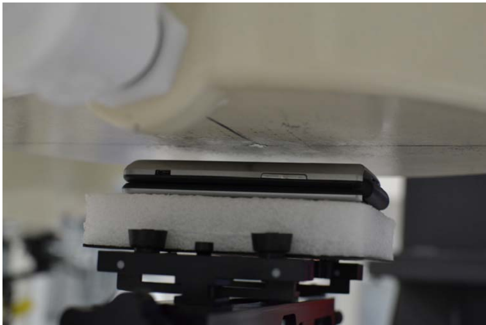
SAR Test Setup Photo 8 Back Side at 10 mm
