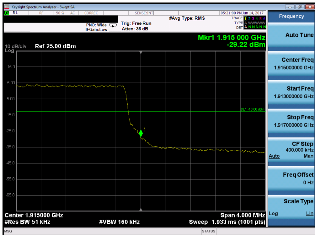
Plot 7-128. Upper Band Edge Plot (Band 25/2 – 5.0MHz QPSK – RB Size 25)
