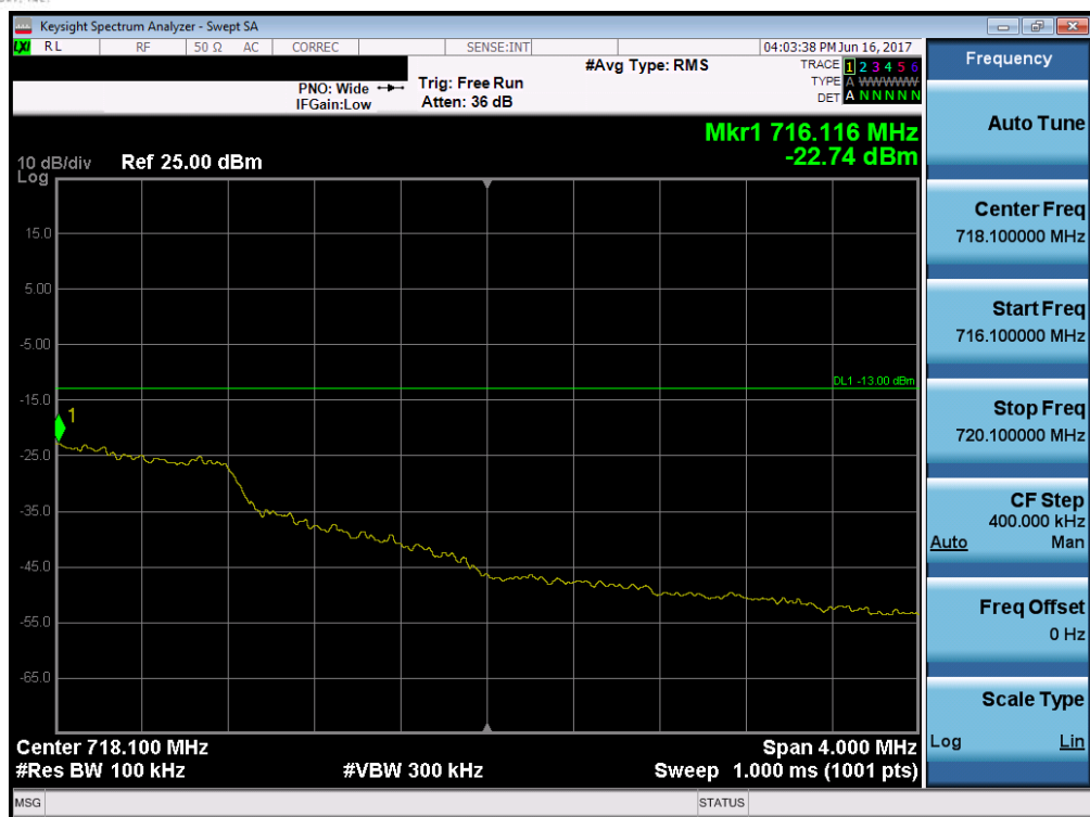
Plot 7-79. Upper Extended Band Edge Plot (Band 12 – 1.4MHz QPSK – RB Size 6)
