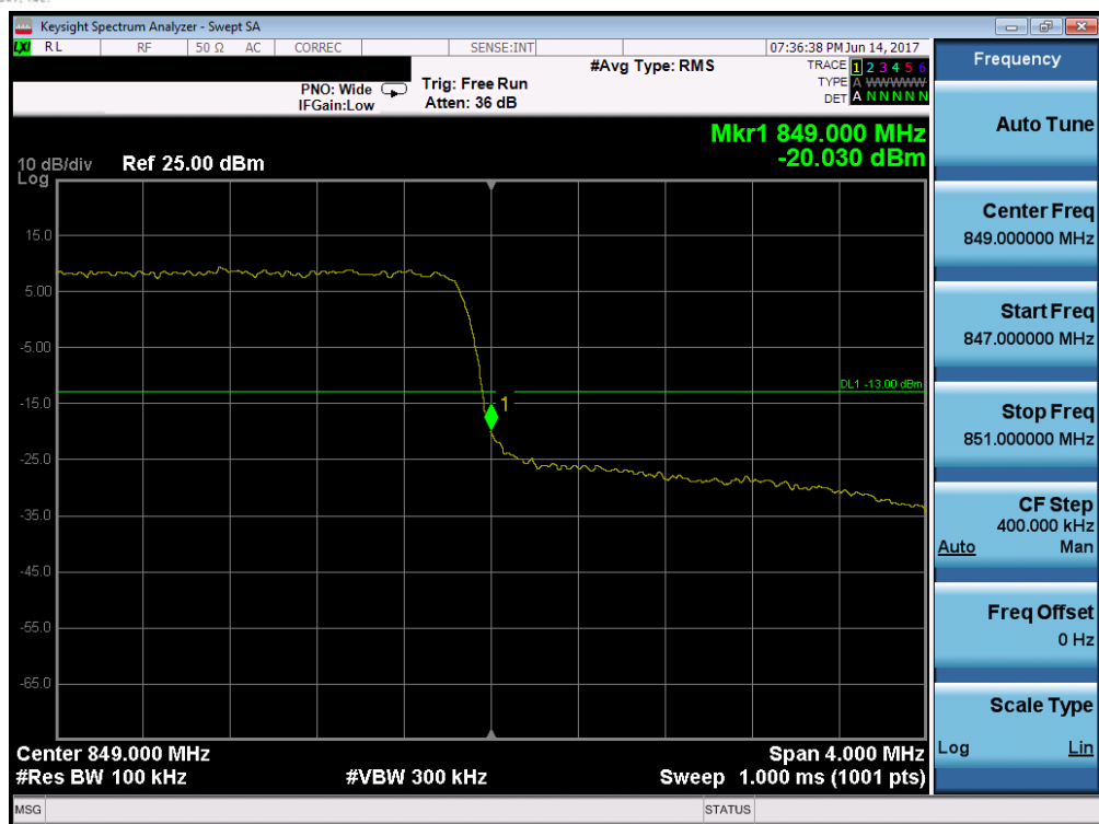
Plot 7-89. Upper Band Edge Plot (Band 5 – 3.0MHz QPSK – RB Size 15)
