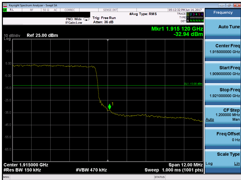
Plot 7-136. Upper Band Edge Plot (Band 25/2 – 15.0MHz QPSK – RB Size 75)
