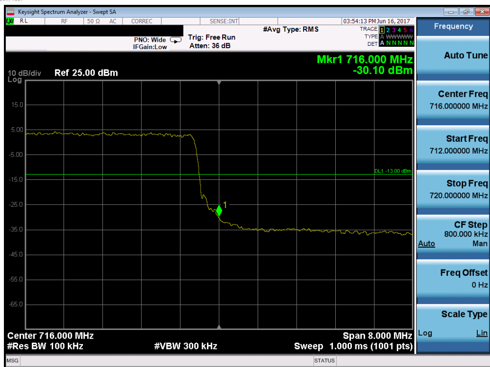
Plot 7-85. Upper Band Edge Plot (Band 12 – 10.0MHz QPSK – RB Size 50)
