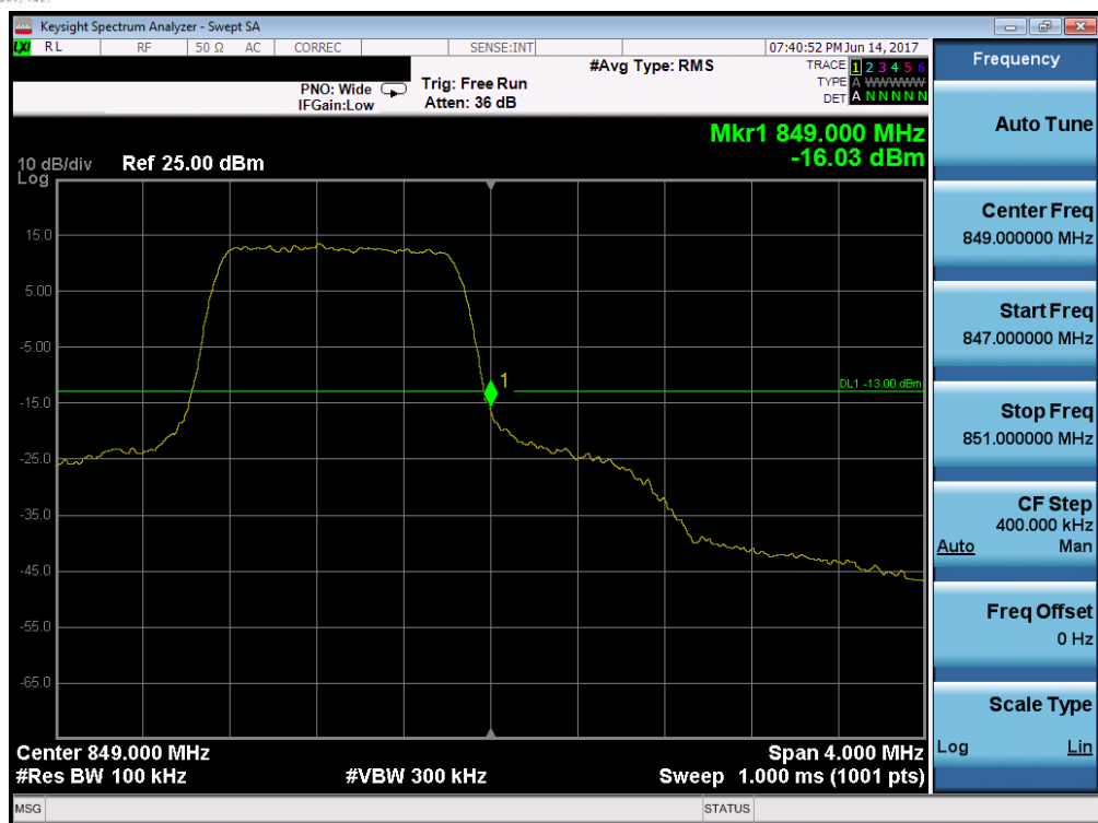
Plot 7-87. Upper Band Edge Plot (Band 5 – 1.4MHz QPSK – RB Size 6)
