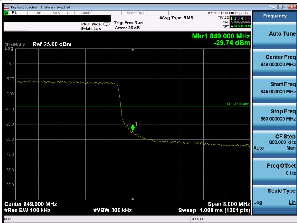
Plot 7-93. Upper Band Edge Plot (Band 5 – 10.0MHz QPSK – RB Size 50)
