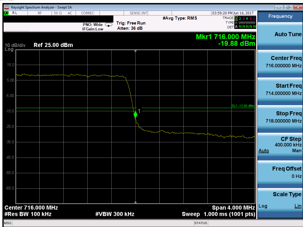
Plot 7-81. Upper Band Edge Plot (Band 12 – 3.0MHz QPSK – RB Size 15)
