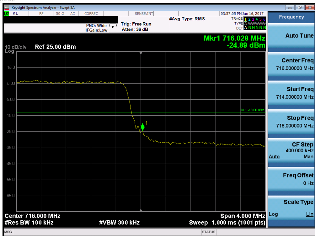
Plot 7-83. Upper Band Edge Plot (Band 12 – 5.0MHz QPSK – RB Size 25)
