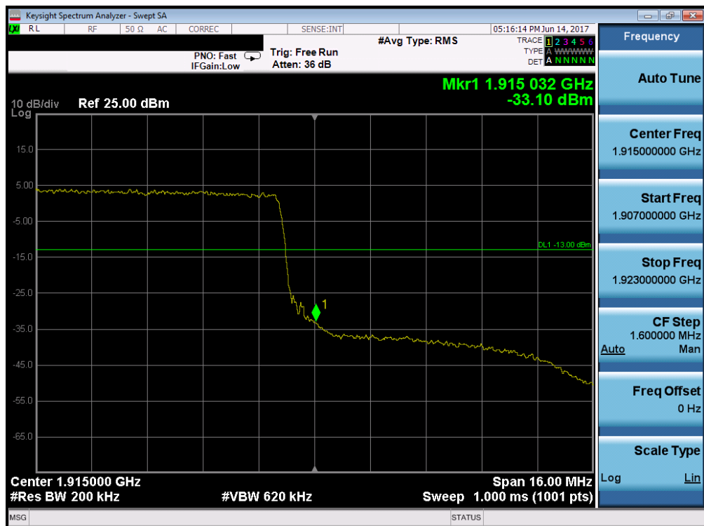
Plot 7-140. Upper Band Edge Plot (Band 25/2 – 20.0MHz QPSK – RB Size 100)
