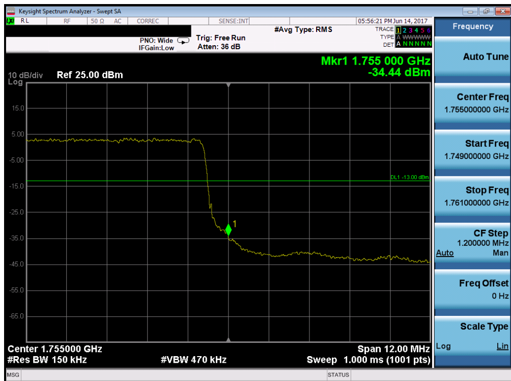
Plot 7-112. Upper Band Edge Plot (Band 4 – 15.0MHz QPSK – RB Size 75)
