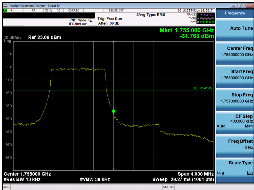
Plot 7-96. Upper Band Edge Plot (Band 4 – 1.4MHz QPSK – RB Size 6)
