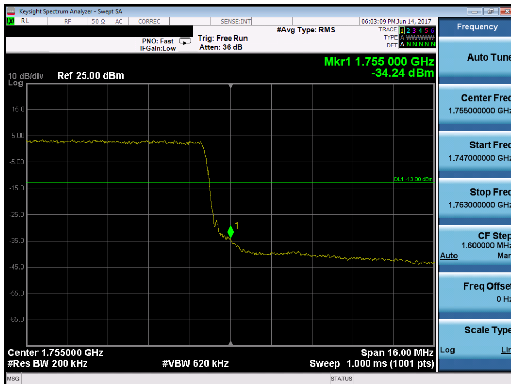
Plot 7-116. Upper Band Edge Plot (Band 4 – 20.0MHz QPSK – RB Size 100)
