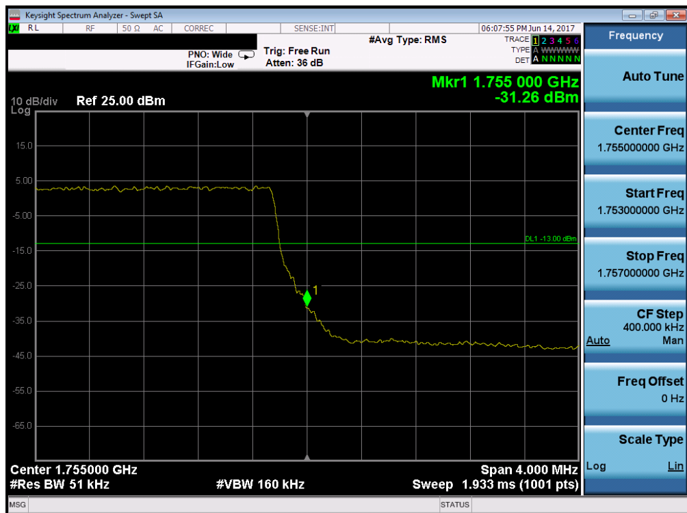
Plot 7-104. Upper Band Edge Plot (Band 4 – 5.0MHz QPSK – RB Size 25)
