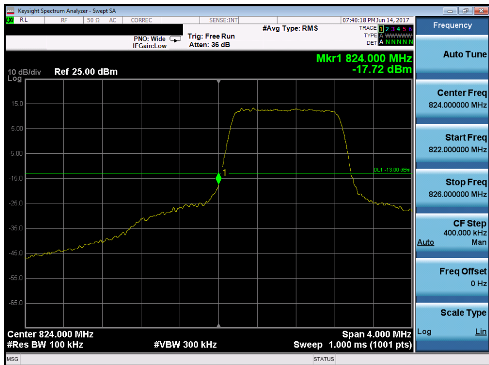
Plot 7-86. Lower Band Edge Plot (Band 5 – 1.4MHz QPSK – RB Size 6)
