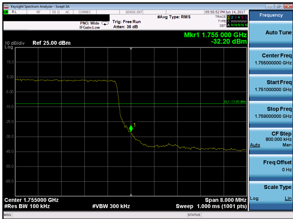
Plot 7-108. Upper Band Edge Plot (Band 4 – 10.0MHz QPSK – RB Size 50)
