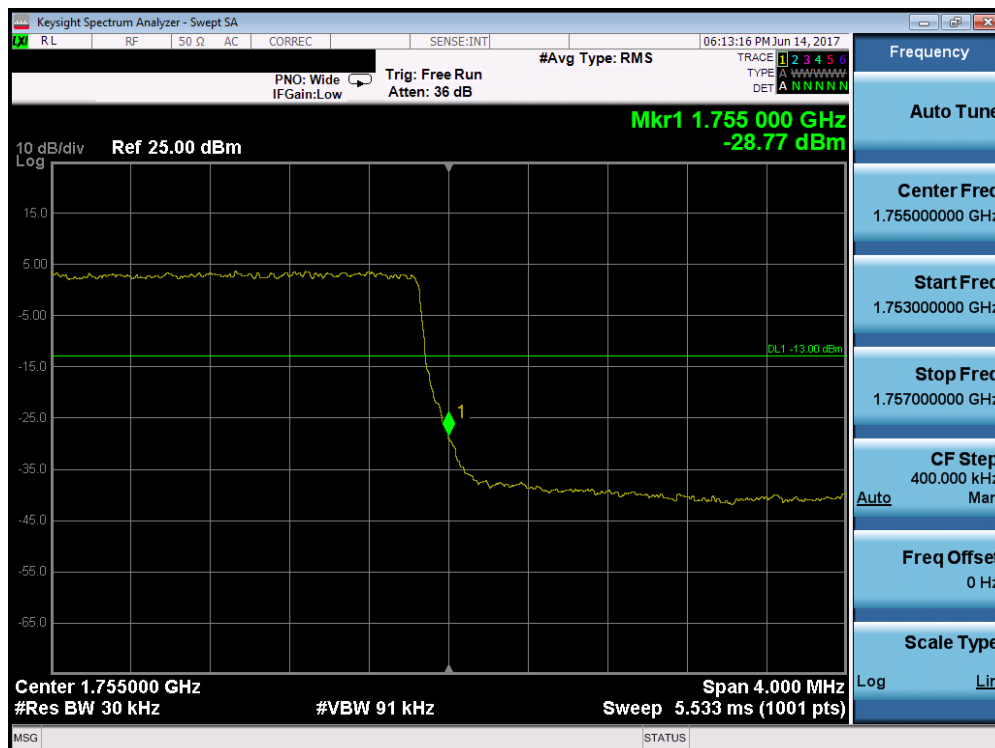
Plot 7-100. Upper Band Edge Plot (Band 4 – 3.0MHz QPSK – RB Size 15)
