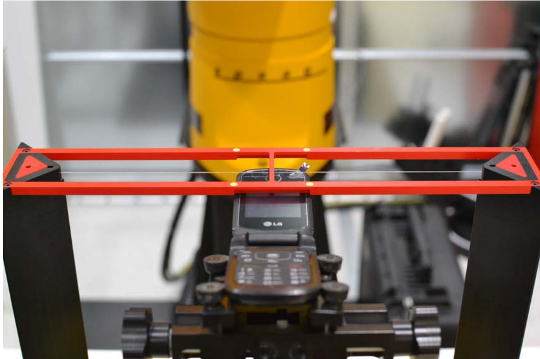
Figure 17-1 Ear Reference Point HAC Phantom Alignment
