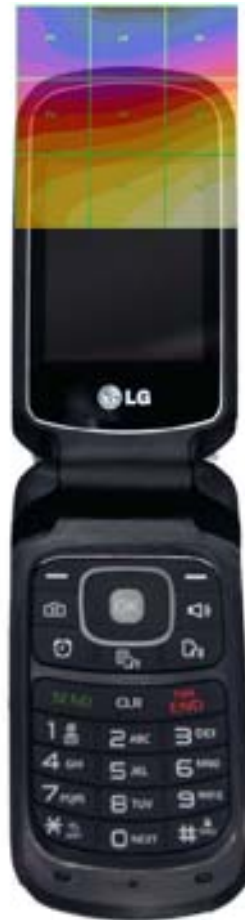
Figure 17-5 H-Field WD Scan overlay
