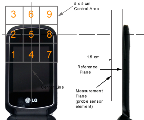
Figure 17-3 5x5 Scan grid above WD
