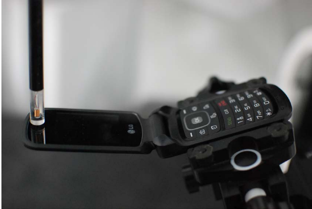
Figure 13-1 Test Setup for Wireless Device
