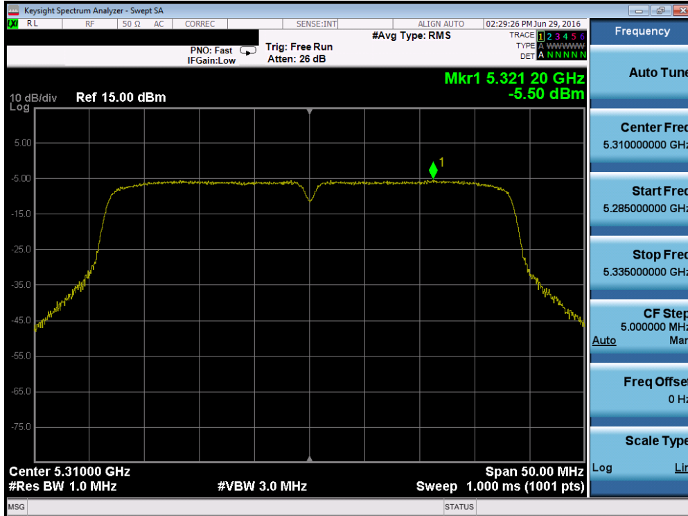
Plot 7-54. Power Spectral Density Plot (40MHz BW 802.11n (UNII Band 2A) – Ch. 62)
