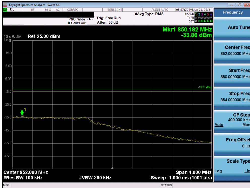
Plot 7-100. Upper Extended Band Edge Plot (Band 5/26 – Band 5 – 3.0MHz QPSK – RB Size 15)
