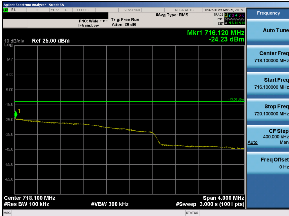
Plot 6-91. Upper Extended Band Edge Plot (Band 12 – 3.0MHz QPSK – RB Size 15)
