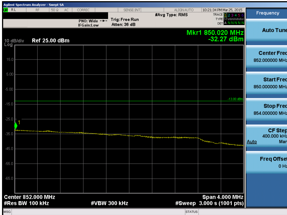
Plot 6-121. Upper Extended Band Edge Plot (Band 5 – 5.0MHz QPSK – RB Size 25)
