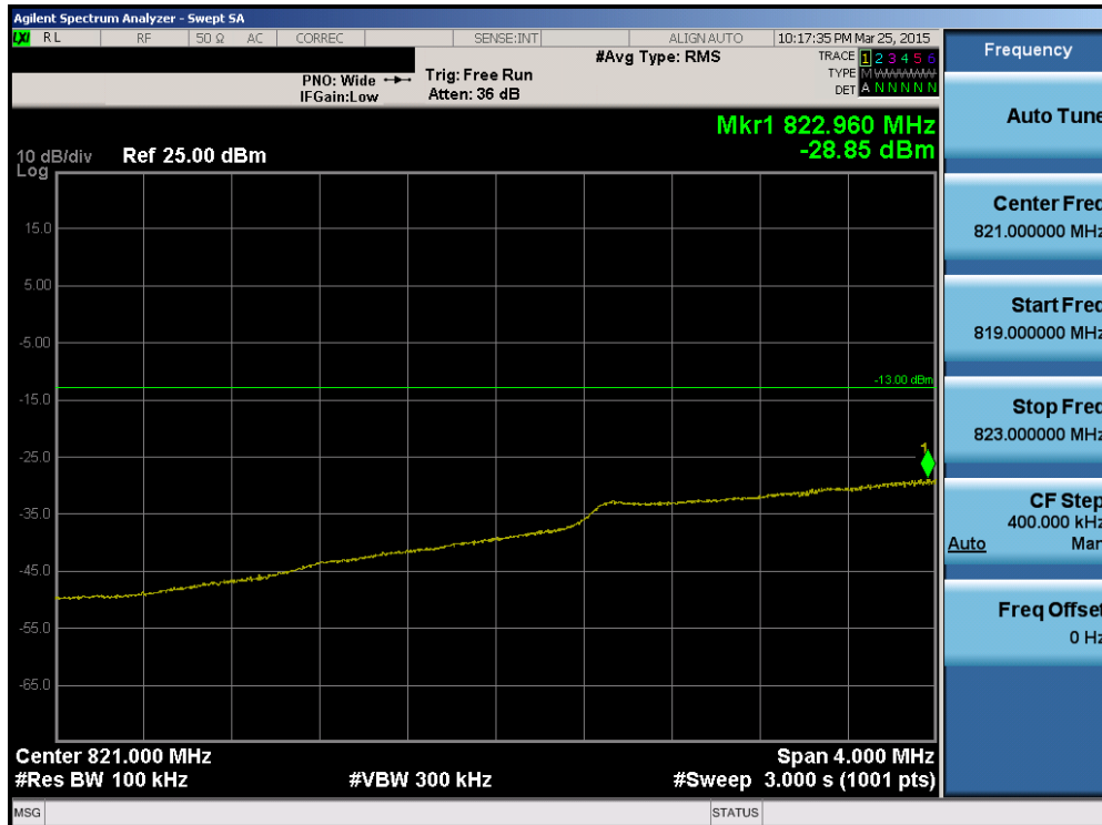
Plot 6-115. Lower Extended Band Edge Plot (Band 5 – 3.0MHz QPSK – RB Size 15)
