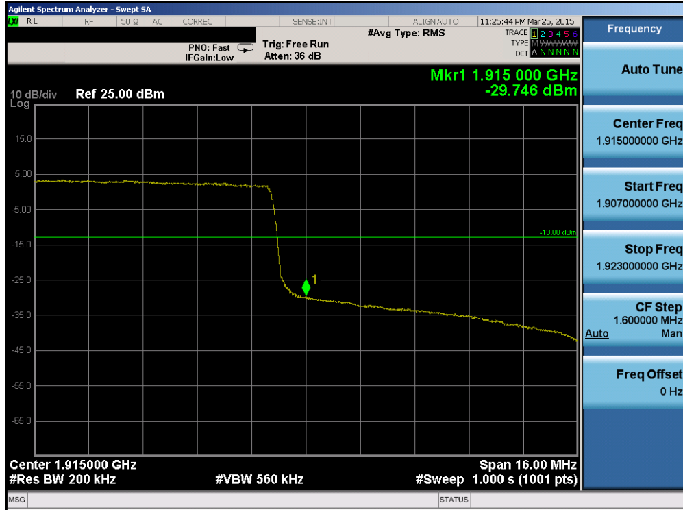
Plot 6-170. Upper Band Edge Plot (Band 25 – 20.0MHz QPSK – RB Size 100)
