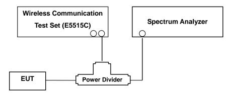
(Configuration of conducted Emission measurement) Test Procedure
