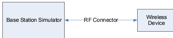
Figure 9-1 Power Measurement Setup
