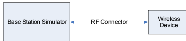
Figure 9-2 Power Measurement Setup
