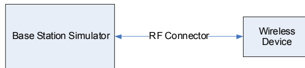
Figure 9-3 Power Measurement Setup
