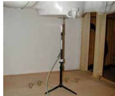
Figure 10-2 System Verification Setup Photo
