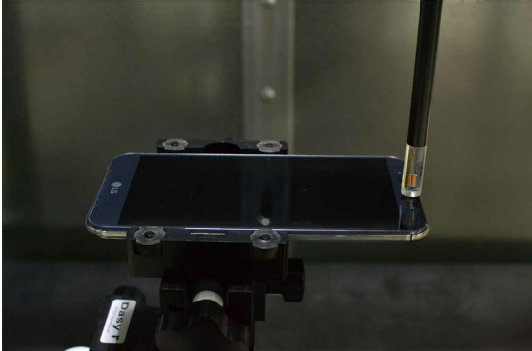
Figure 13-1 Test Setup for Wireless Device
